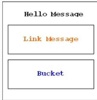
Figure 4.24. OLSR HELLO message Bucket Data Unit encapsulation.
