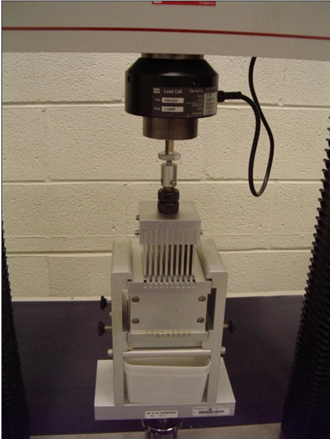
Figure 3.5 Kramer Shear Unit attached to universal testing machine in this research
