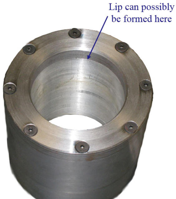
Figure 4-30. By machining the inner bore as an assembly, no lip is formed at the joint between the Upper Plate and the Inner Shell (photo by Ryan Cavey)
