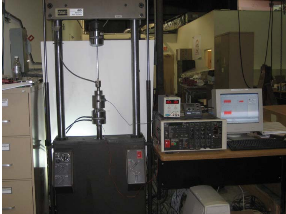
Figure 5-3. The rheometer assembly clamped in the MTS load frame is ready for testing (photo by Ryan Cavey)
