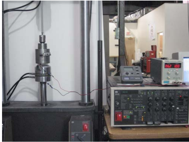
Figure 4-47. The rheometer installed in the load frame ready for testing (photo by Ryan Cavey)
