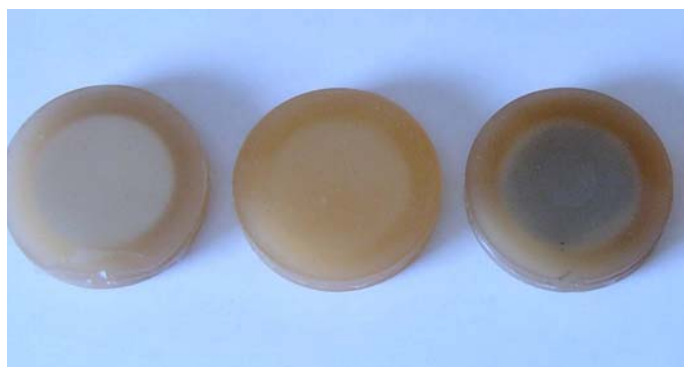
Figure 3-11. Photograph of MR fluid-elastomer vibration isolator specimens (adapted from [3])
