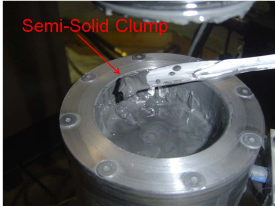
Figure 5-52. A pea-sized aggregate clump that has formed in the MR fluid test chamber (photo by Ryan Cavey)
