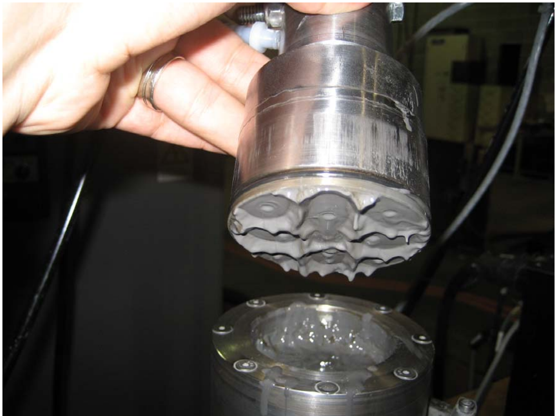
Figure 5-61. Semi-solid clumps form around multiple sites in the Multi-hole Piston (photo by Ryan Cavey)
