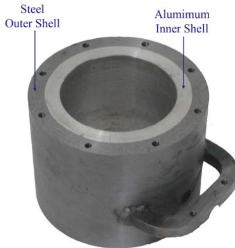
Figure 4-29. The Inner and Outer Shells pressed together (photo by Ryan Cavey)
