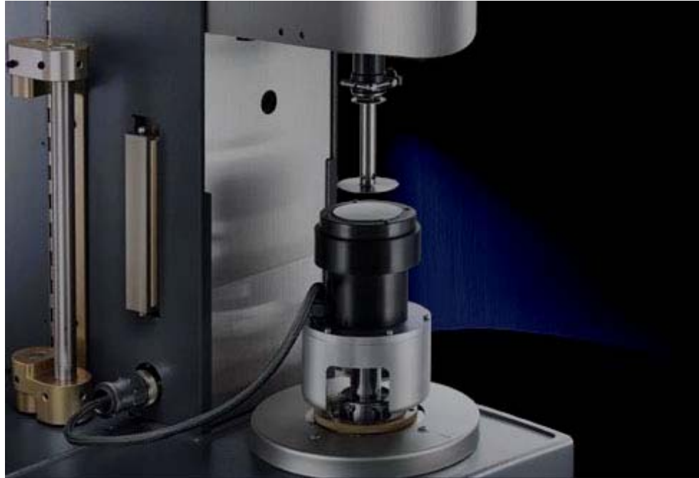
Figure 4-1. A typical rotational shear-type rheometer from TA Instruments (image adapted from [45])
