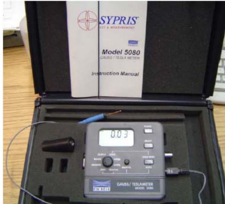
Figure 4-44. Gauss-meter and “ultra-thin” transverse probe (image adapted from [51])
