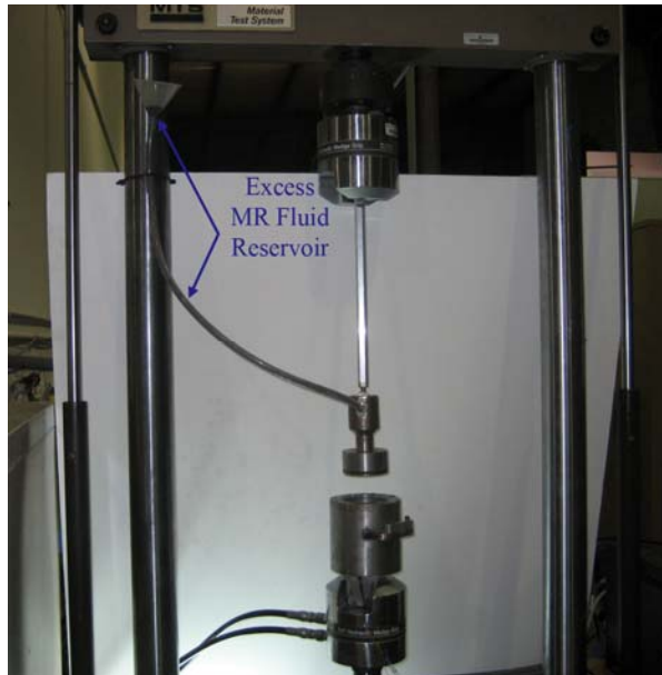
Figure 5-9. The reservoir for excess MR fluid is kept above the test chamber to allow air to escape (photo by Ryan Cavey)
