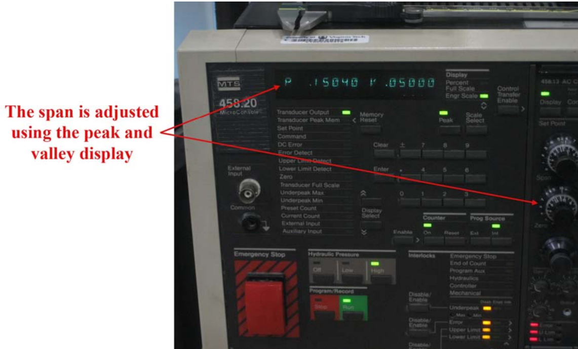
Figure 5-6. The fine adjustment of the span is performed while the actuator is in motion (photo by Ryan Cavey)
