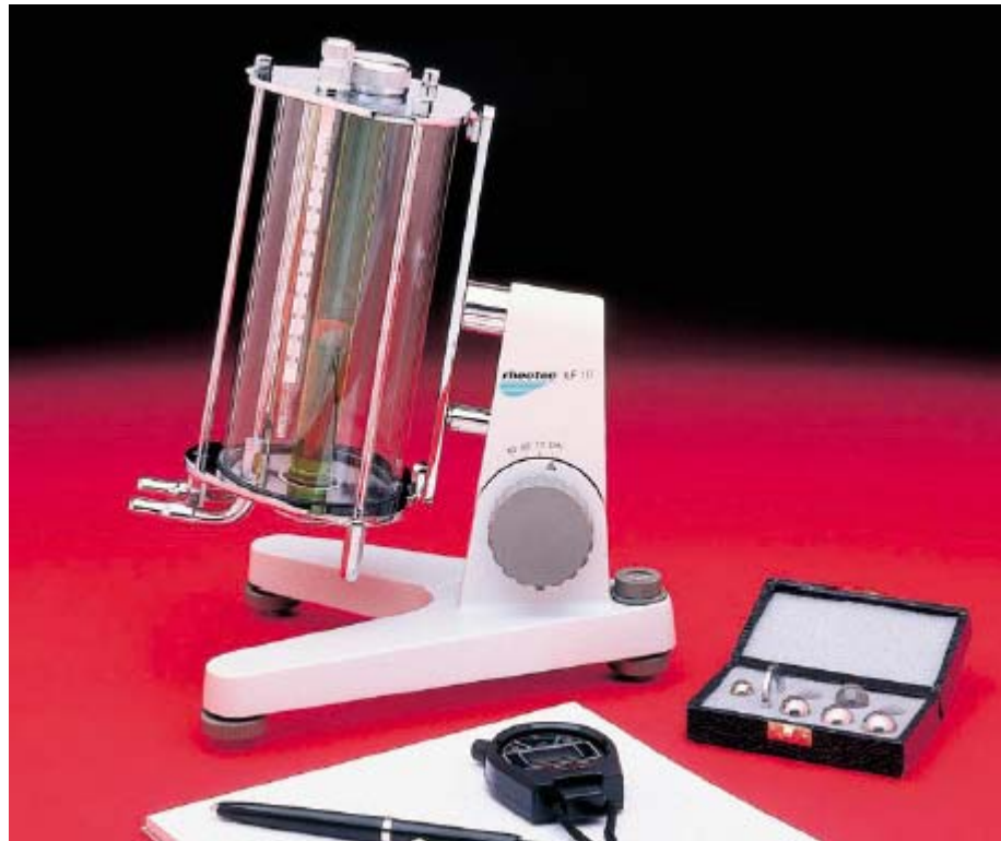
Figure 4-3. A falling ball rheometer from RheoTec Messtechnik GmbH (image adapted from [46])
