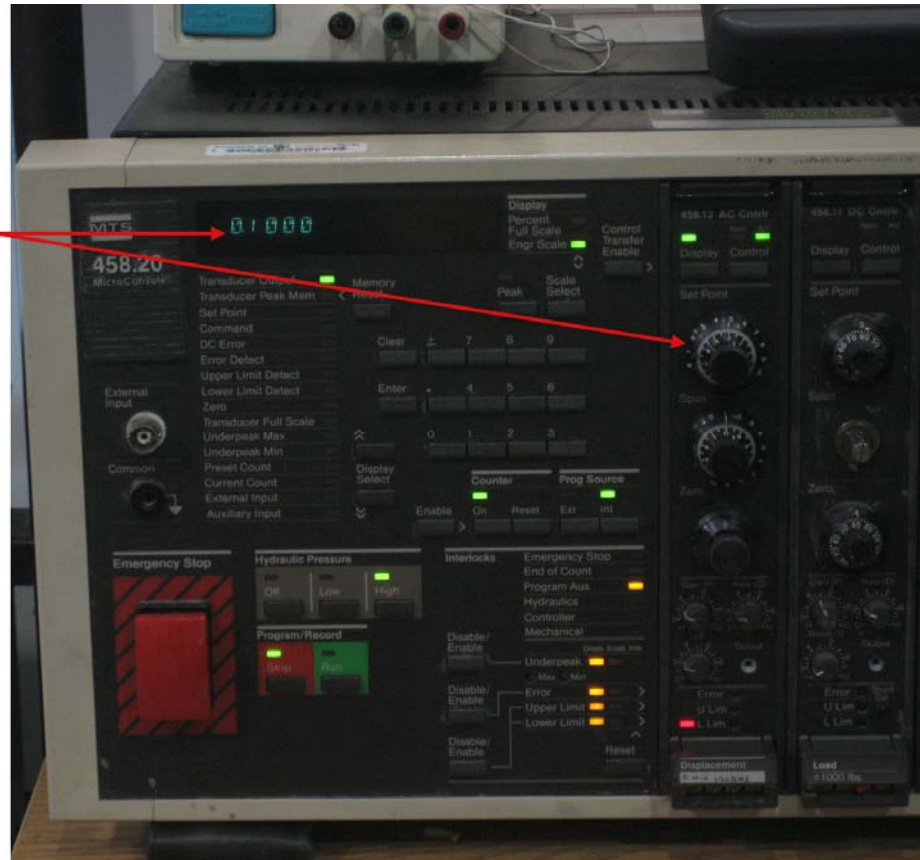
Figure 5-5. The Set Point marks the center point of the ramp wave used for testing (photo by Ryan Cavey)
