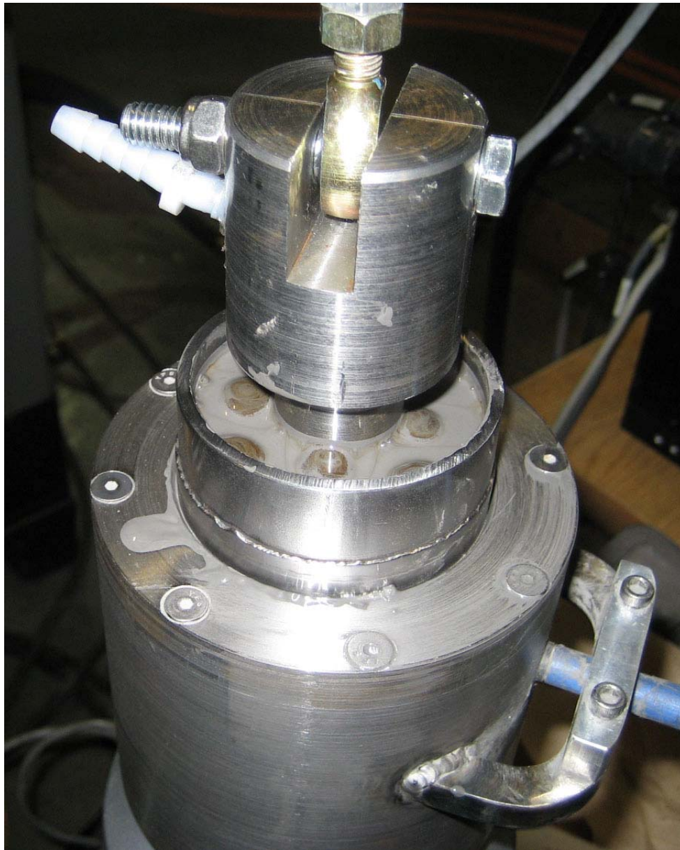
Figure 5-62. Columns of separated carrier fluid appear to form directly over the eight thru holes in the piston (photo by Ryan Cavey)
