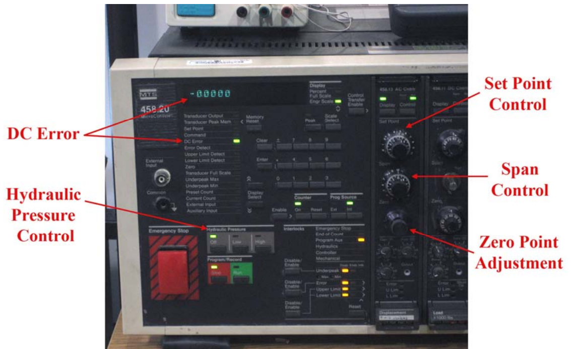
Figure 5-4. Controls for the MTS 458 controller (photo by Ryan Cavey)
