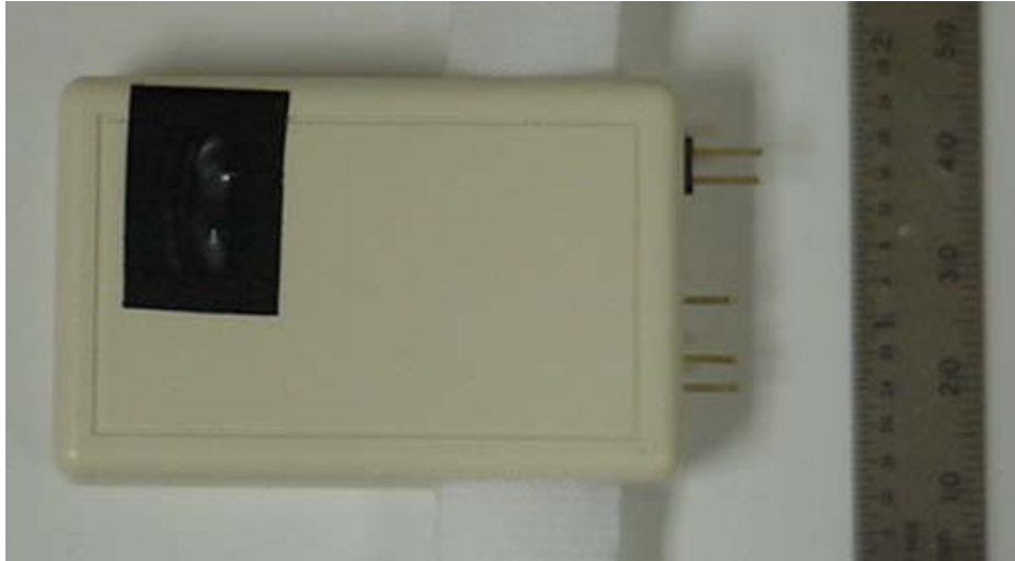
Figure 3.6.3. Bottom view of the outside of the acceleration measurement device housing.
