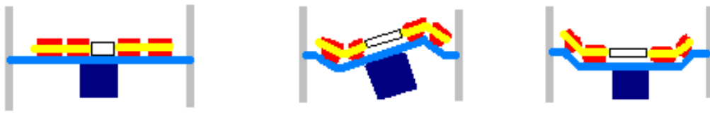
Figure 3.2.2.2. Piezoelectric accelerometer interior during static vertical gravity (left), an XY acceleration (middle), and a vertical acceleration (right).
