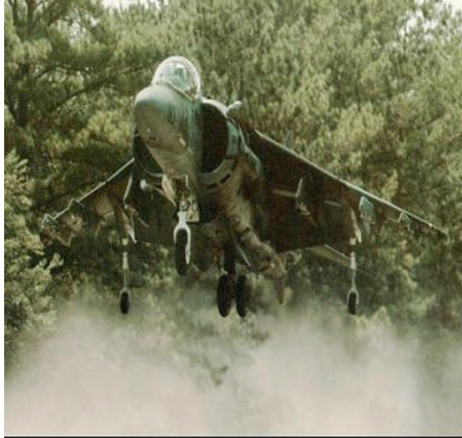
Figure 1-1: The AV-8B Harrier on take off is an example of hot exhaust gases mixing with cooler atmospheric air [www.globalsecurity.com].
