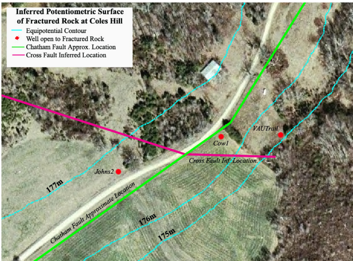
Figure 4.13: Inferred potentiometric surface of fractured rock aquifer at the south spring area of Coles Hill.
