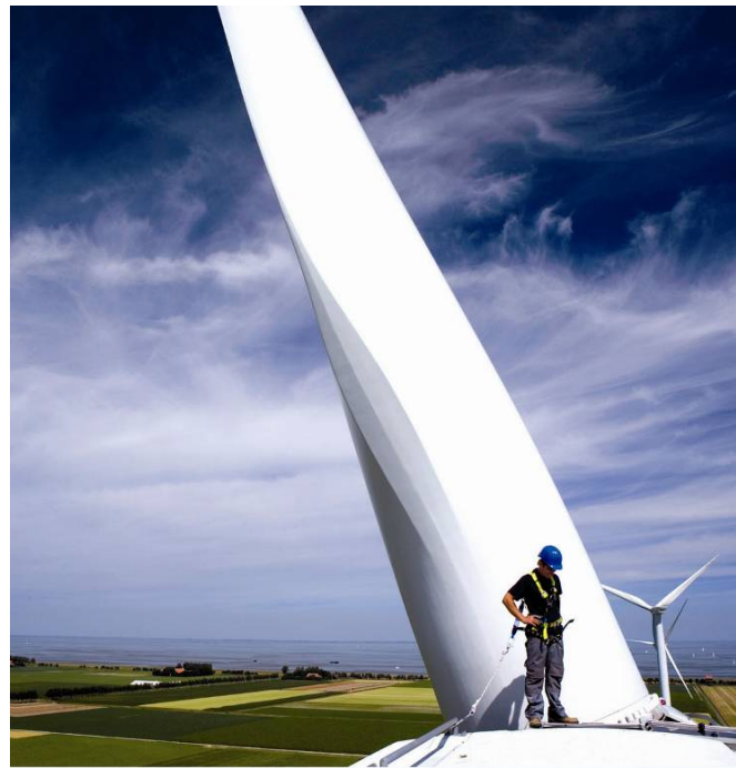
Figure 1.5: Root region of a modern large wind turbine's blade. It can be observed the region in which the airfoil's shapes used have large blunt trailing edges. This region is located in the transition between the circular sections of the root and the typical aerodynamic sections of the rest of the blade. (Used with permission of Jack Mowry, Editor, Sound & Vibrations Magazine, March 2008 and LMS international)
