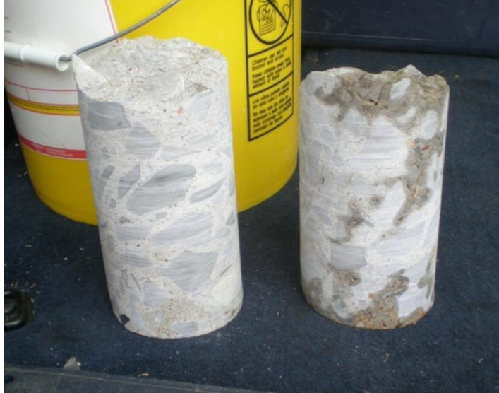
Figure 5-2. Extracted Concrete Sample Cores
