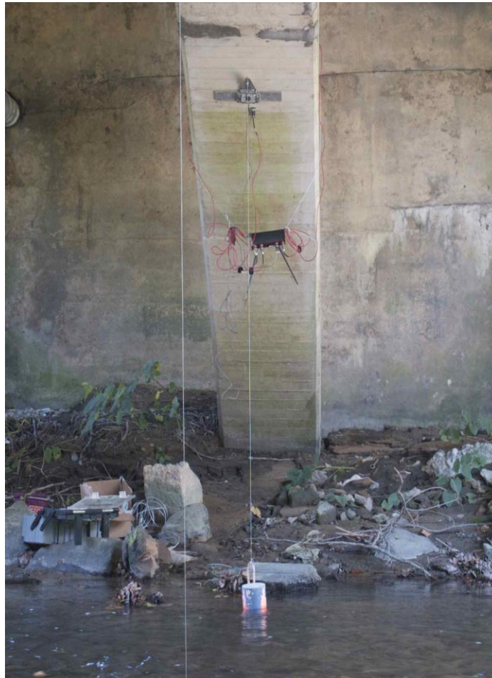
Figure 3-3. Deflectometer Attached to Weight
