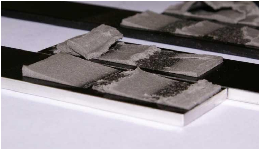
Figure 2.27 Representative failed shear VHB tape specimens, tested at 23°C (73°F), showing wedge-shaped residual adhesive.
