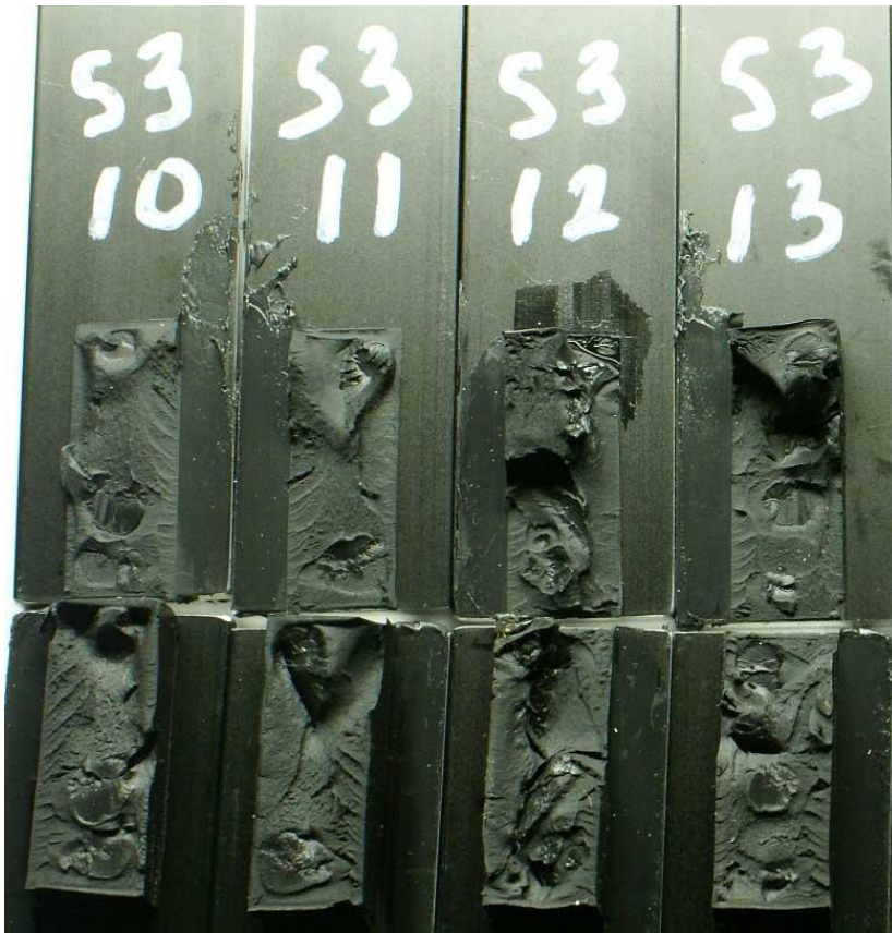
Figure 2.40 Failed S3 shear creep rupture specimens.
