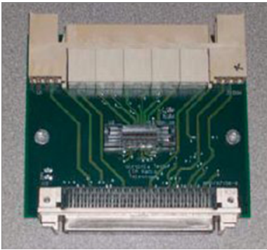
Figure 5.1: ML310 to S25 and EDT interface adapter board. top: ML310 connection, middle: MICTOR to S25 connection, bottom: EDT connection.
