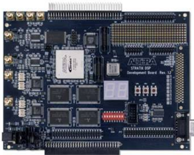
Figure 3.8: The Altera Stratix DSP development board (S25) used as the digital receiver nodes in the ETA radio telescope.
