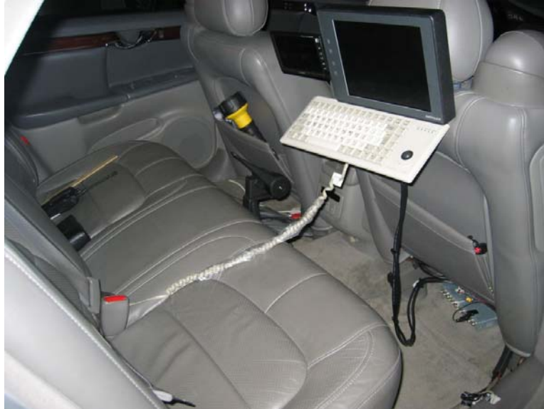
Figure 3.12: Experimenter data collection interface.
