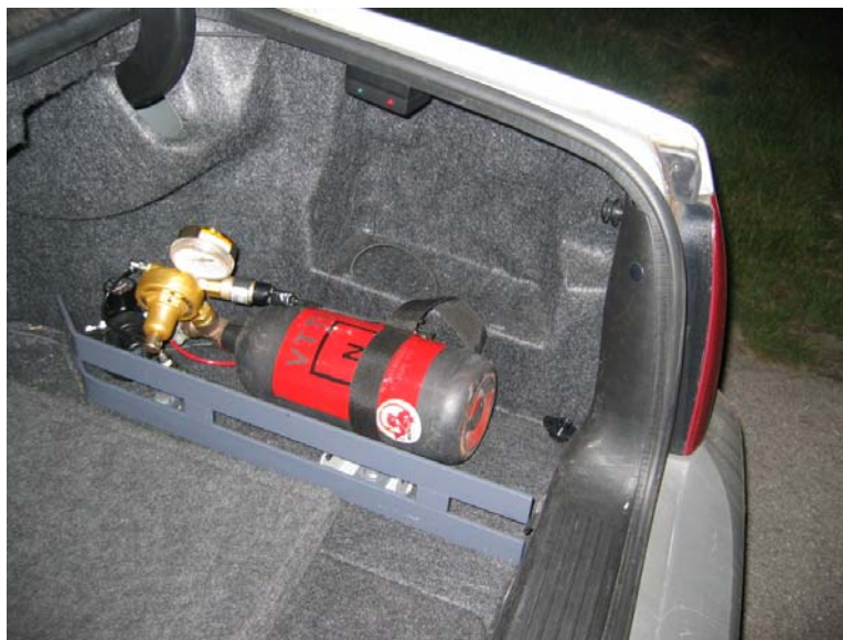
Figure 3.10: Nitrogen tank located in trunk used to power throttle push-back as well as emergency brake.
