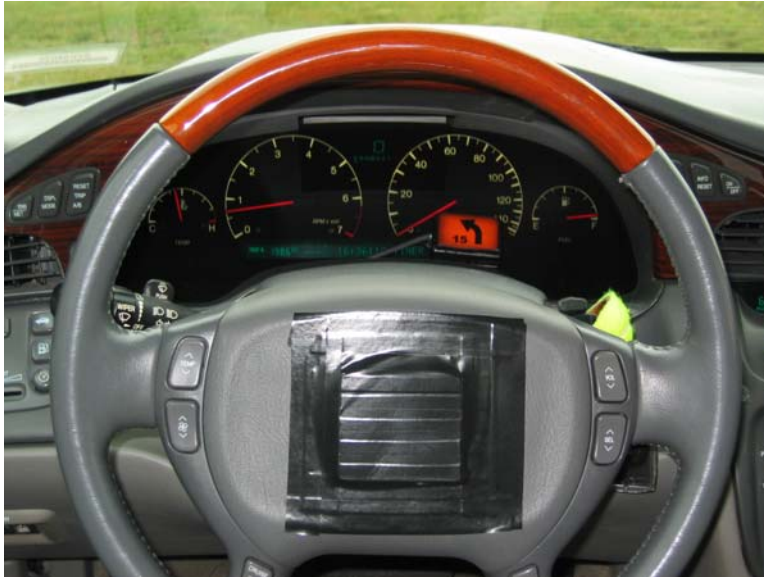
Figure 3.2: HDD location on dash.
