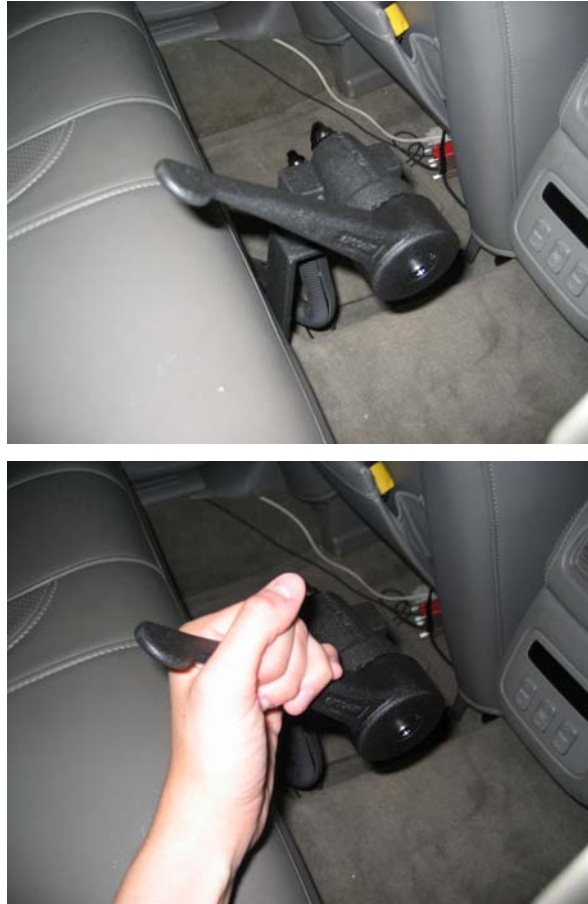
Figure 3.9: Custom-built hand brake accessible to backseat passenger.
