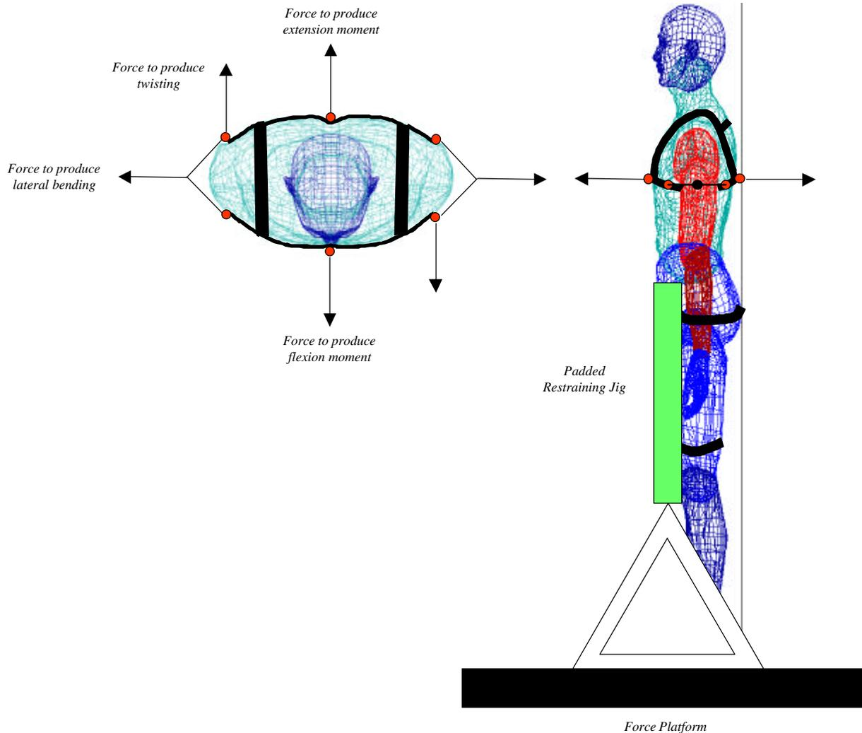
Figure 1. Data Collection Apparatus
