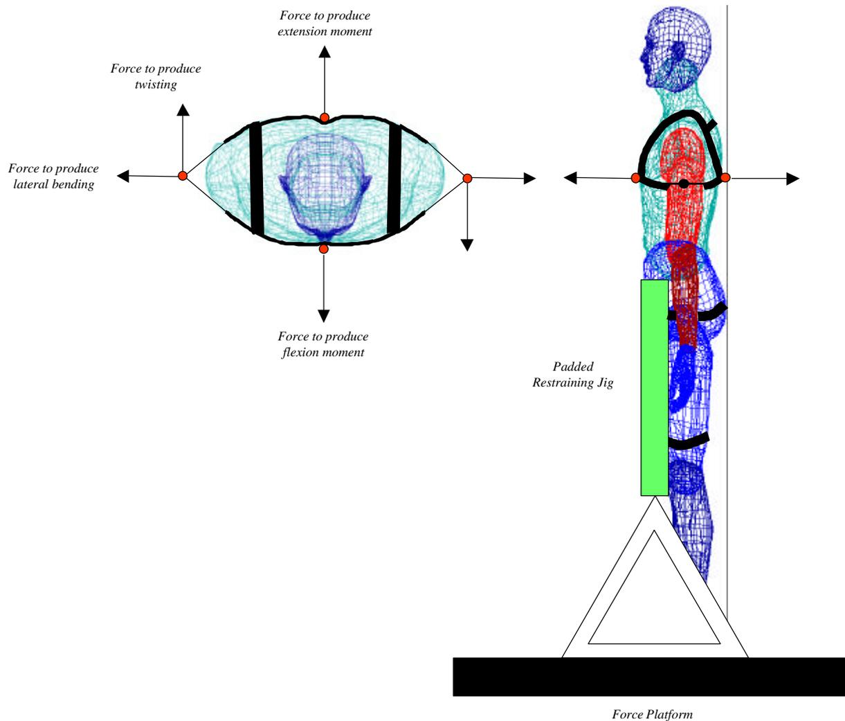
*Figure 6. Experimental setup. Red circles are load attachment points. The forces will be generated through vertical loads redirected through pulleys and attached to the harness via cables.*
