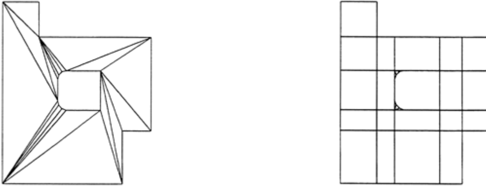
Fig 5-2 Correct Modeling for desirable Tessellation
