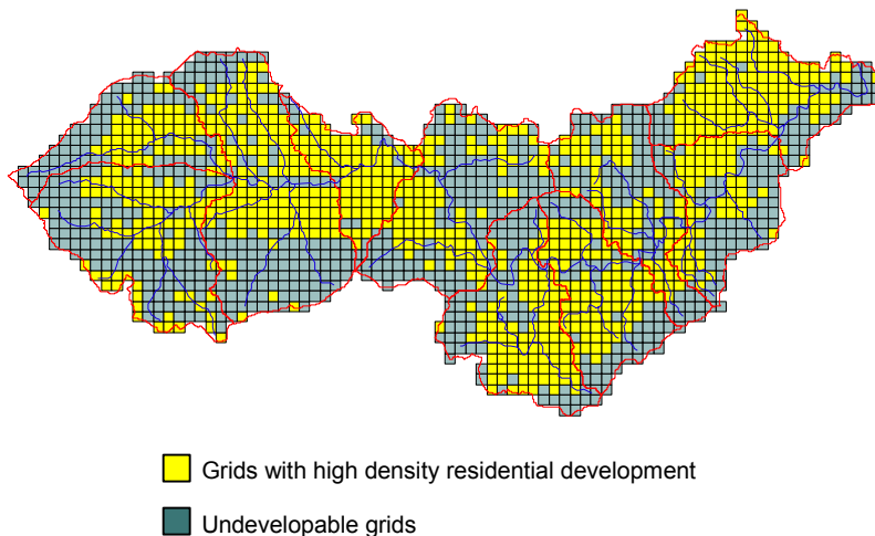
Figure 4.1. High density development in the entire watershed (Development Scenario I) 12
