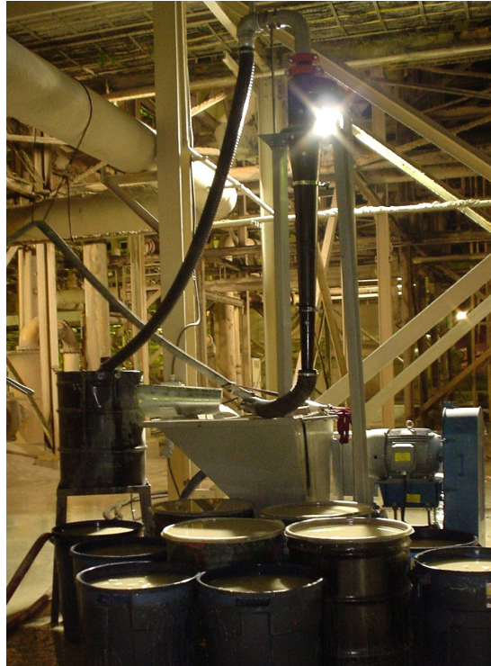
Figure 3.2. Hydrocyclone Set-Up for Slimes Collection.
