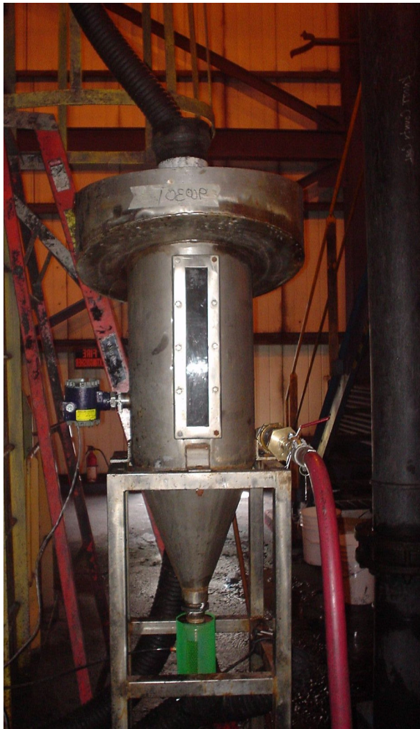
Figure 2.13. Pilot-Scale HydroFloat Separator Test Circuit at Plant B.
