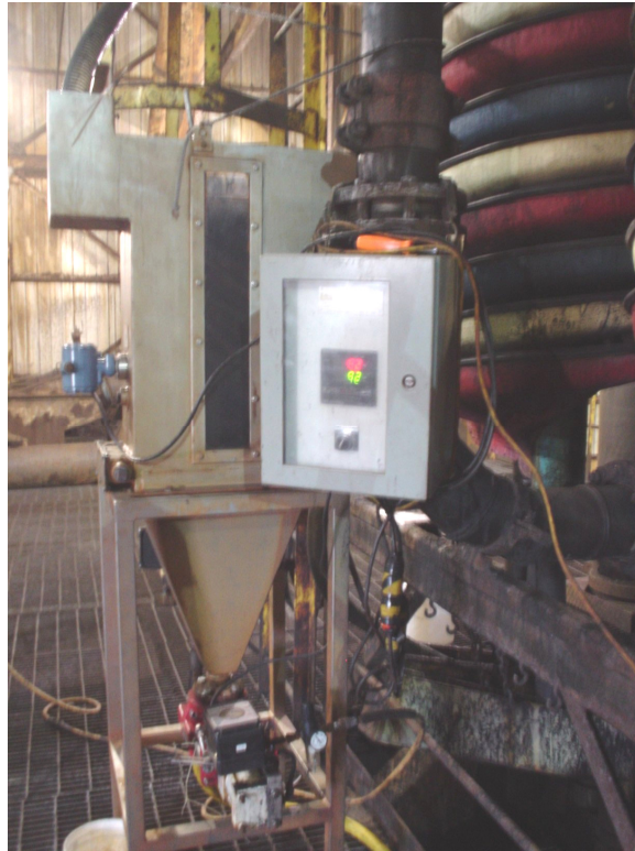
Figure 1.7. The 9x16 Inch Pilot-Scale Crossflow Test Circuit at Coal Plant B.
