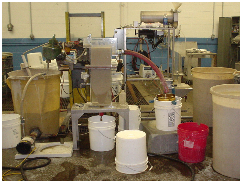
Figure 3.3. Laboratory CrossFlow Unit (2x6 Inch) Utilized for Sample Concentration.
