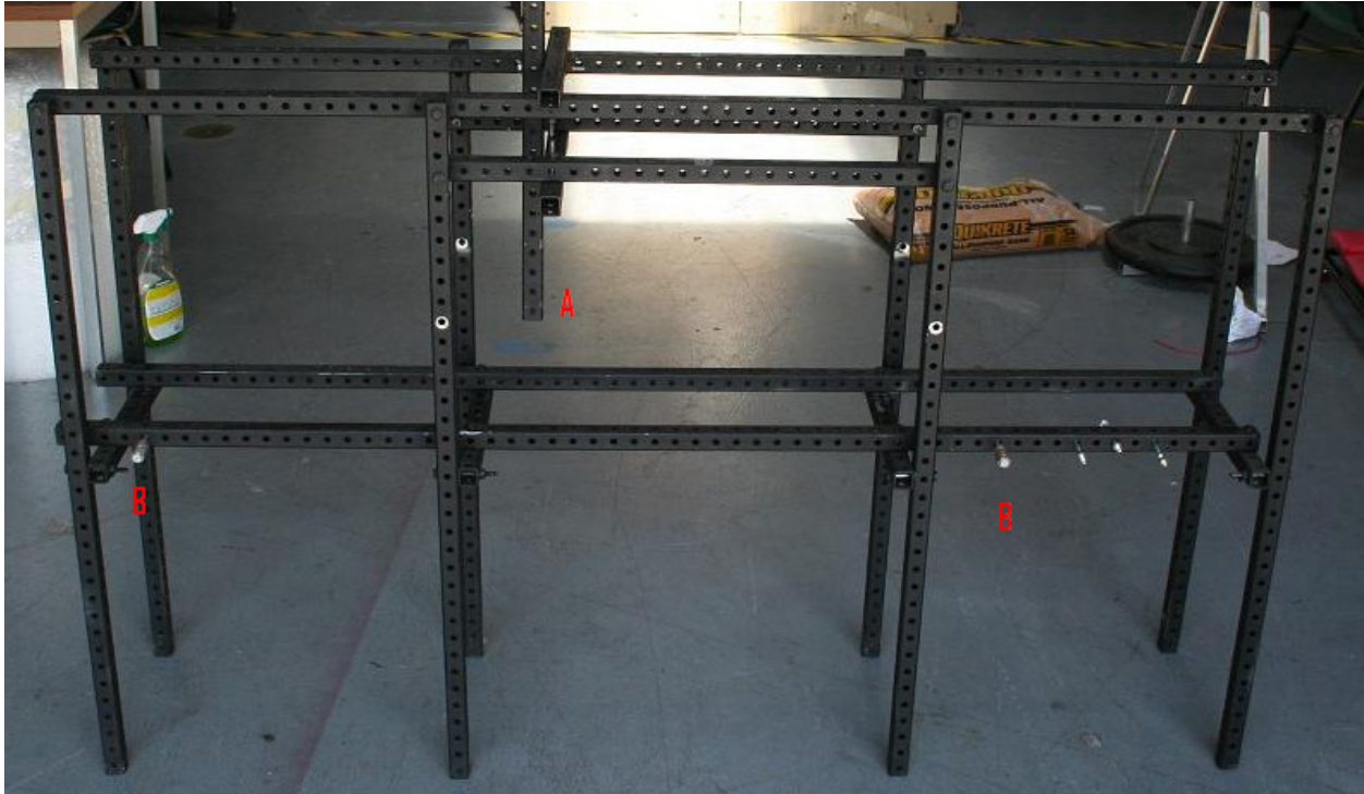
Figure A-1. Support structure for welding experimental setup. A – welding arm, B – guide screws. The welding torch secures to the welding arm so that it remains in a fixed position, and the guide screws are used to ensure that the slide table moves the target in a
