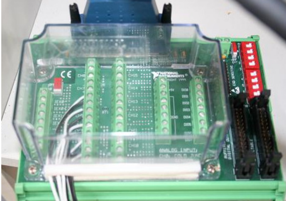
Figure A-13. TBX-68T temperature/voltage logger. The black and white wires connected to the TBX-68T carry voltage signals from the thermocouple modules to their respective channels.
