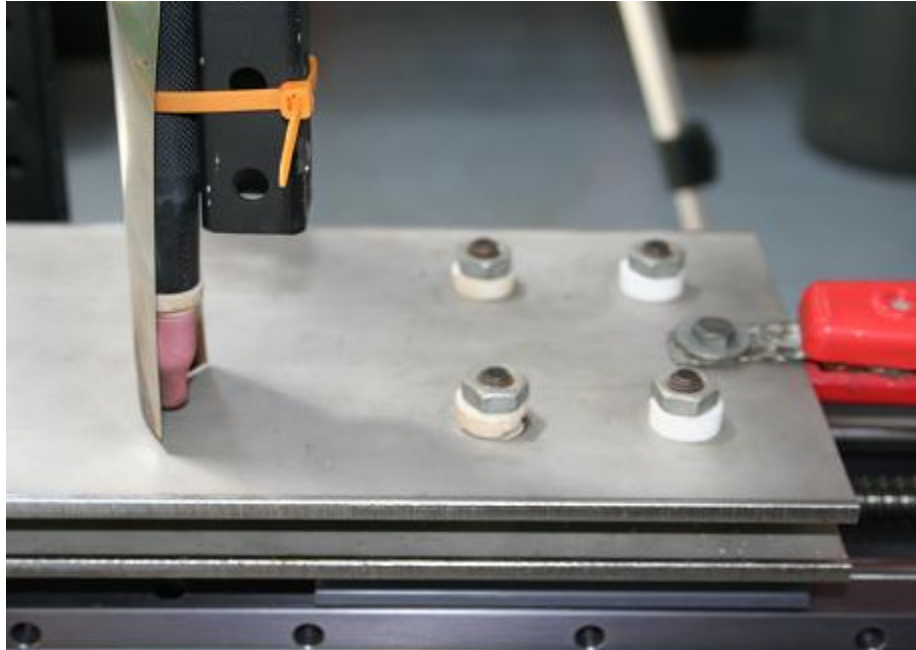
Figure A-11. Support end of completely installed target plate. Also visible are the welding torch and welding shield, both of which are secured to the welding arm of the support structure with standard zip ties. The welding safety plate is also visible below the target plate.
