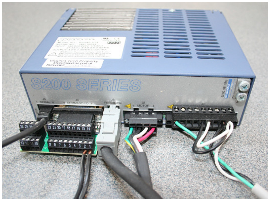
Figure A-6. Close up of S200 series servo driver showing all connections.
