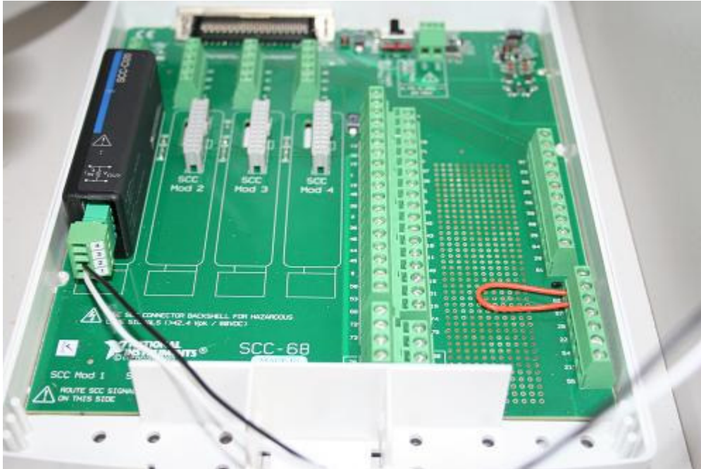
Figure A-14. SCC-68 multifunction DAQ device and SCC-CI20 current input module. Also shown are terminals 62 and 67 with an orange jumper wire connecting them.
