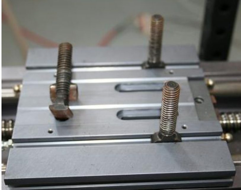
Figure A-8. Slide table carriage and T-slot bolts.
