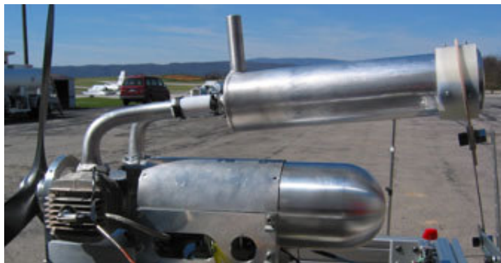
Figure 3.21: Picture of the 2-1 silencer mounted on the twin cylinder engine.
