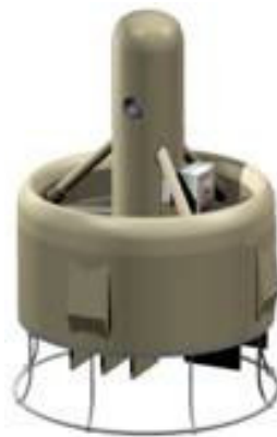
Figure 1.3: The prototype Allied Aerospace VTOL UAV vehicle.
