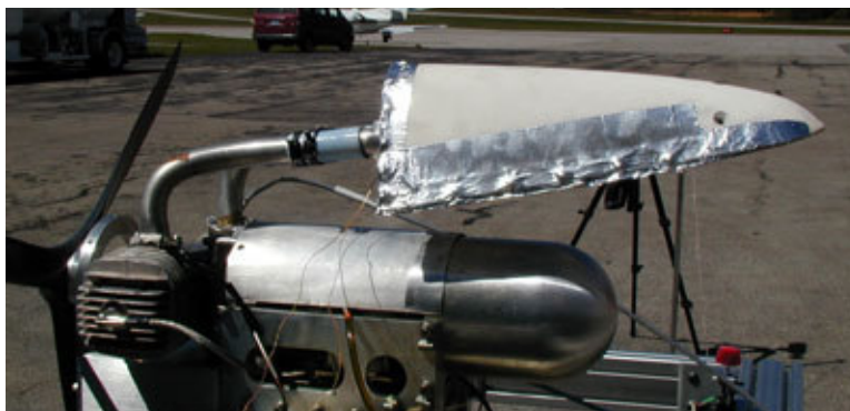
Figure 3.33: Picture of the aerodynamic shell w/ 3-hole foam mounted on the twin cylinder engine.
