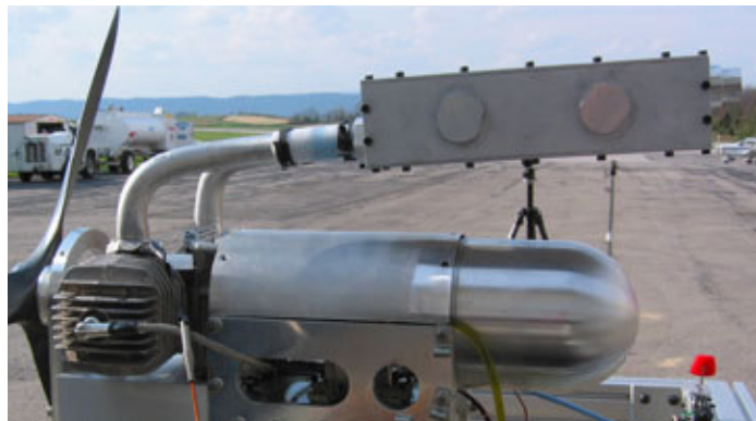
Figure 3.25: Picture of the expansion box mounted on the twin cylinder engine.
