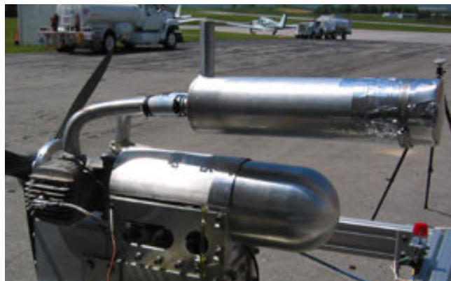
Figure 3.23: Picture of the 2-1 silencer w/ foam mounted on the twin cylinder engine.
