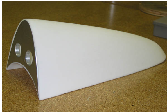
Figure 3.32: Picture of the SLS shell before refractory foam was added.
