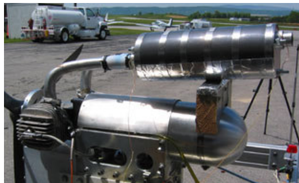
Figure 3.30: Picture of the nylon cylinder w/ 3-hole foam mounted on the twin cylinder engine.
