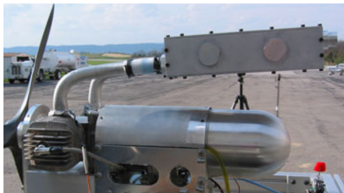
Figure 3.27: Picture of the box w/ 3-hole foam mounted on the twin cylinder engine.
