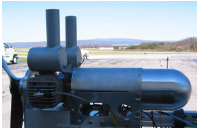
Figure 3.15: Picture of single exit twins mounted on the twin cylinder engine.
