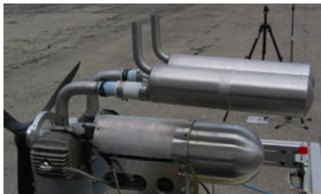
Figure 3.19: Picture of the long twins mounted on the twin cylinder engine.
