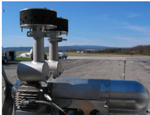
Figure 3.17: Picture of single exit twins w/ diffusers mounted on the twin cylinder engine.
