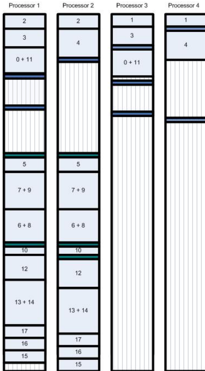
Figure 6.6: Example schedule for boost rectifier application
