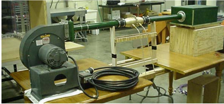
Figure 3.23. The experimental setup used a blower to introduce a known flow rate into the enclosure instead of using the system fans.
