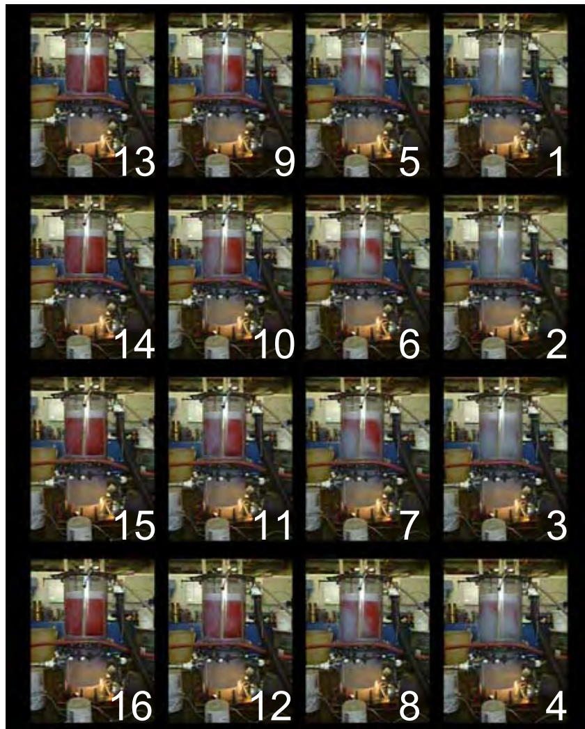
Figure 15. Visualization of column mixing using a red dye and timed-sequence images at one-second intervals.
