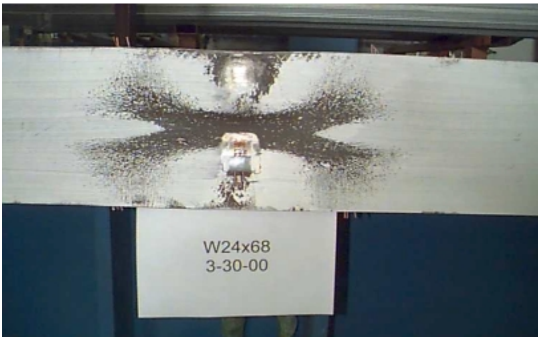
FIGURE 3-3. Yield Line Pattern Observed Throughout the Five Specimens (View of Bottom Flange from Below After Test)
