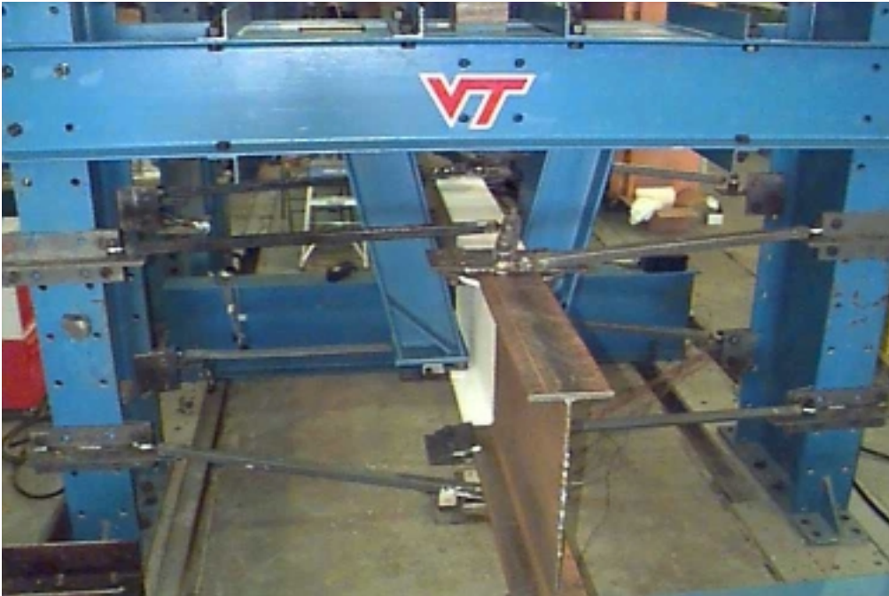
FIGURE 2-1. Test Set-up during the First Phase of the Research
