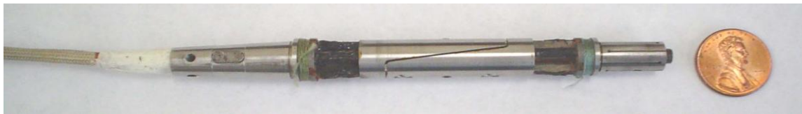
Appendix Figure B-3: Close-up of the GA-11 balance.
