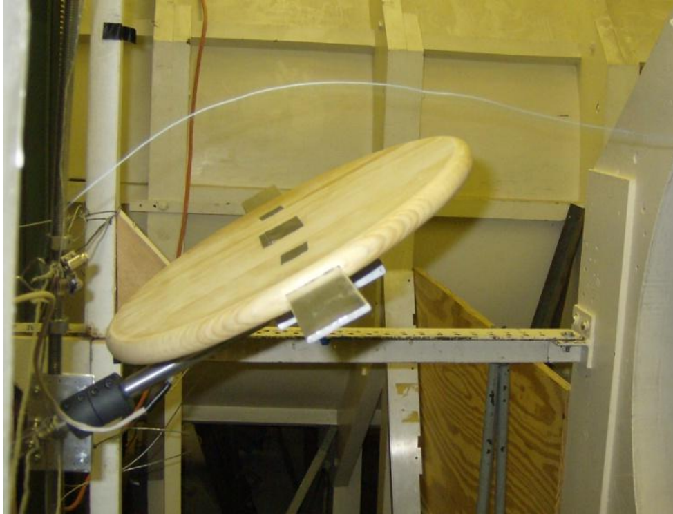
Figure 3-4: Low Reynolds Test with Blades Extended in Open-Jet Tunnel.
