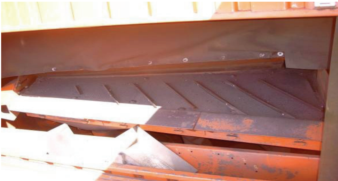
Figure 3.7 Air-table deck (1 m 2 ) of pilot scale dry deshaling unit.
