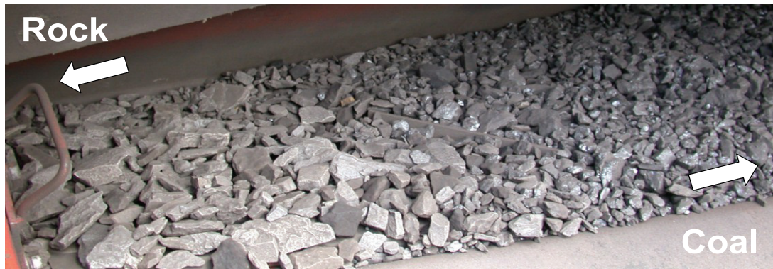
Figure 2.5 Segregation of coal and rock along the length of the vibrating air table.
