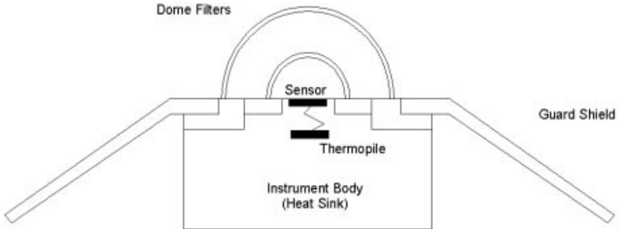
Figure 1.1 The pyranometer
