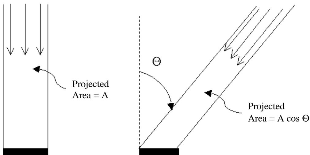
Figure 1.3 Cosine-law response of the sensor surface
