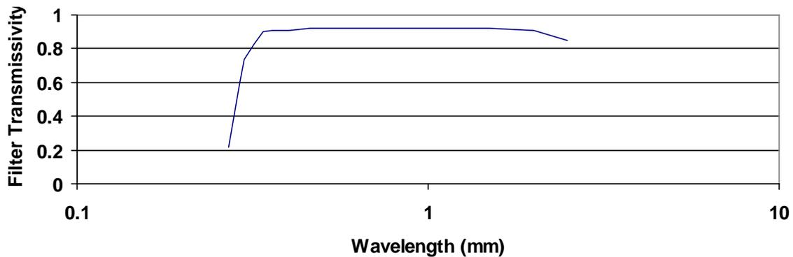
Figure 1.2 Filter function for Schott glass 2.0-mm dome filter
