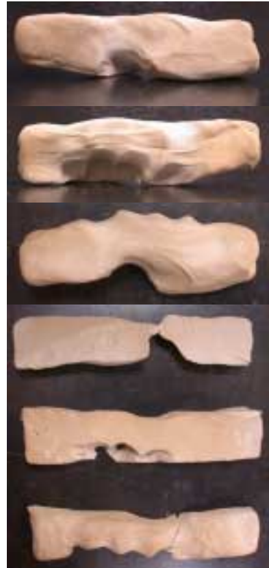
Impression of a hand made by grasping a clay extrusion similar to the extruded arm of an aluminum standard walker frame.
