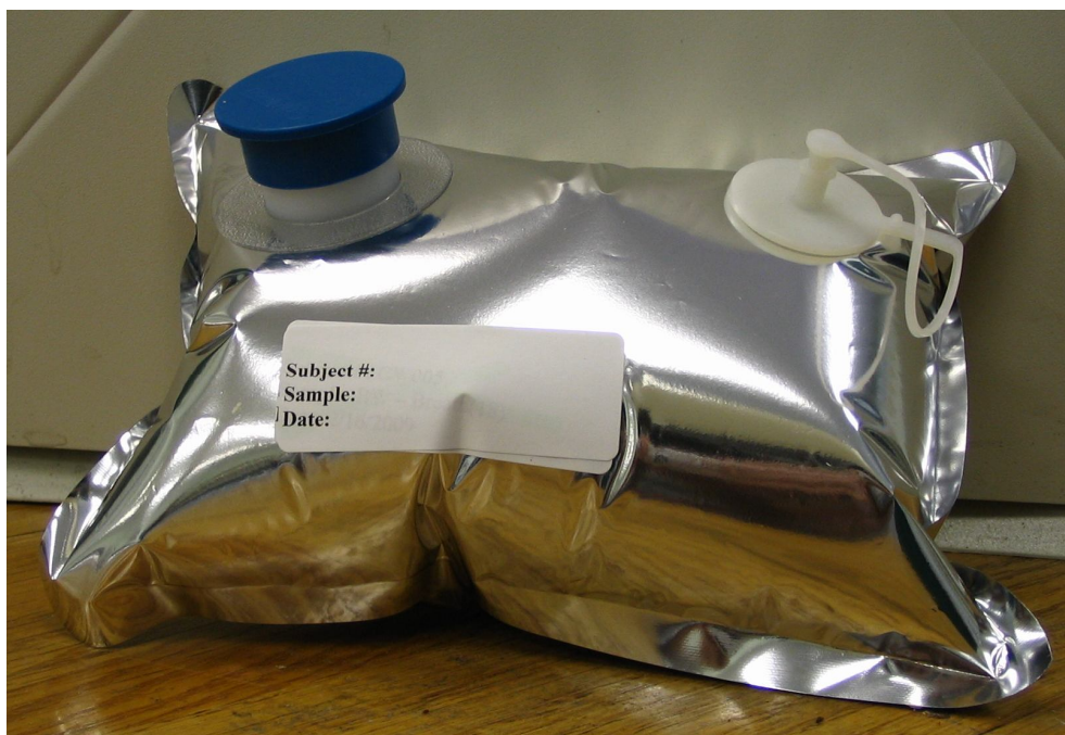
Figure 3.3. Breath samples were collected in an alveolar air collection device and stored for up to 10 hours in the collection bag.
