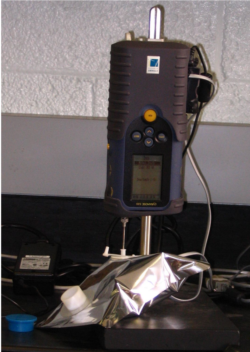
Figure 3.4. The C320 snout is inserted into the luer port to analyze the breath sample.
