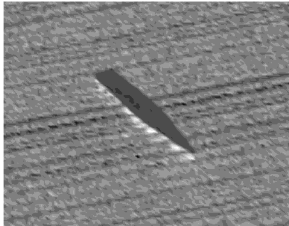
Figure 4.23 The change in infrared contrast produced when using a vertical polarization filter ( \epsilon = 0.85 , r^s = 0.1 , \theta = 50 deg, T_{\text{sea}} = 290 K, T_{\text{ship}} = 290 K)
