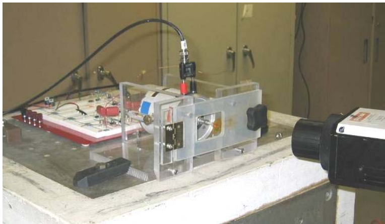
Figure 2.27 Bending test setup for a sensitivity comparison. Photograph by David Griffiths 2/22/2007
