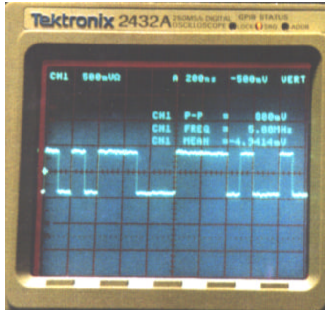
Figure 4.1-7. This signal was measured at the output of the PN sequence generator on the sliding correlator measurement system. The hardware produces the PN sequence with an eleven-stage shift register tapped at [9,11].
