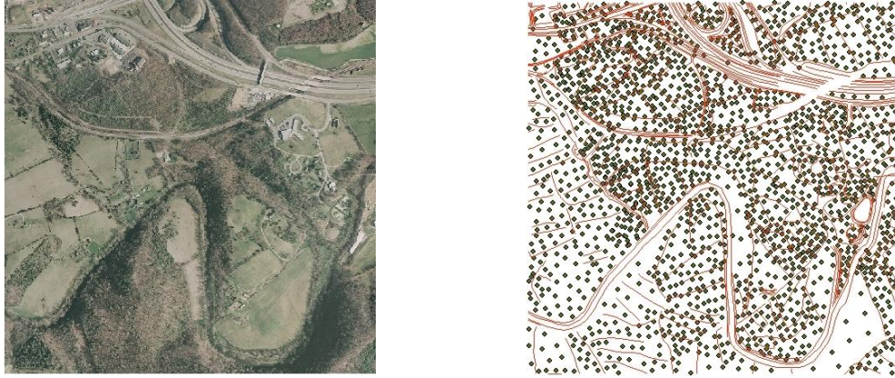
Figure 23 - Aerial photo (left) and masspoints with breaklines (right) from the Virginia Base Mapping Program near Wytheville, VA.
