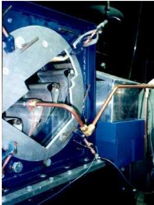
Figure D.5 The pipe with cooling air blowing into the blade.
