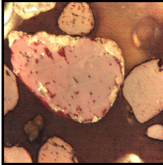
FIGURE 7: RUTILE GRAIN SHOWING BOTH REDDISH BROWN INTERNAL REFLECTIONS AND LAMELLAR TWINNING
