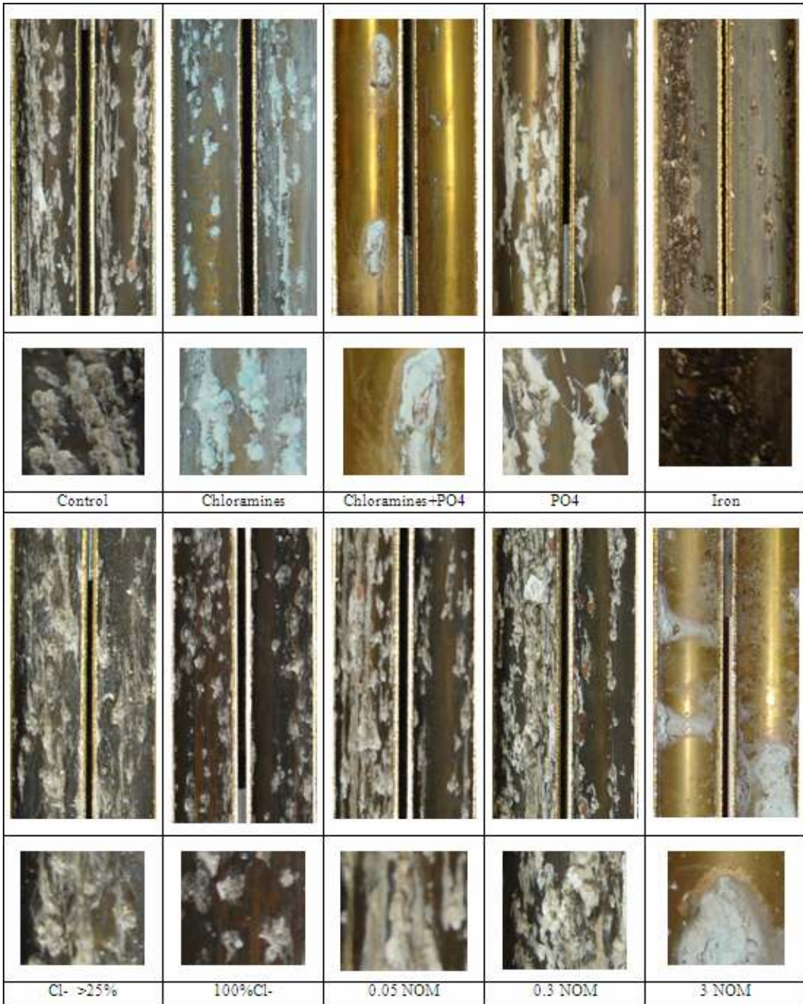
Figure 2.5: Brass photos after 15 months, after raising pH and Cl 2 :NH 4 concentration ratio.
