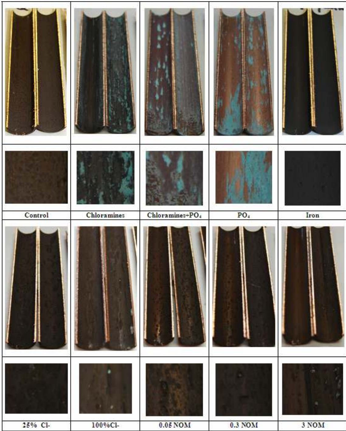
Figure 1.7: Copper type M after the last 3 months and removal of the other metals.
