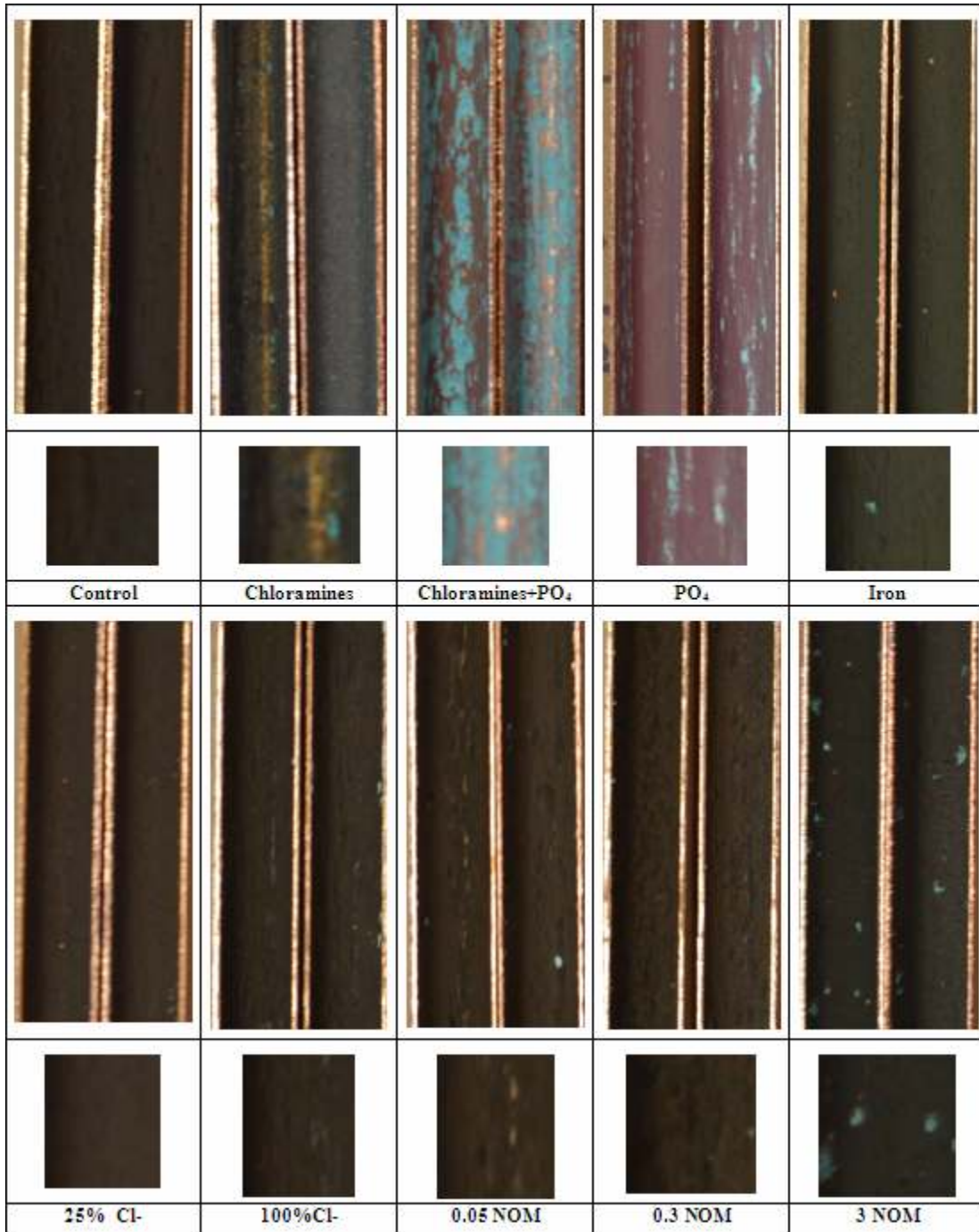
Figure 1.6: Copper type M for the last 5 months after all metals other than copper were removed from the rig.
