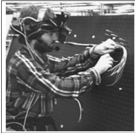
FIGURE 22: Augmented Reality in Boeing's Manufacturing Process [Boeing, 1996]
