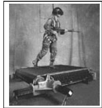
FIGURE 15: VSD Inc.’s Omni-Directional Treadmill [ http://www.vsdevices.com/ ]
