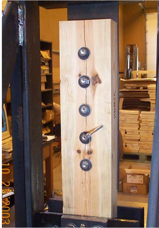
Figure 4.5: Typical Expected Yield Mode III Connection under Monotonic Loading, 6D spacing.
