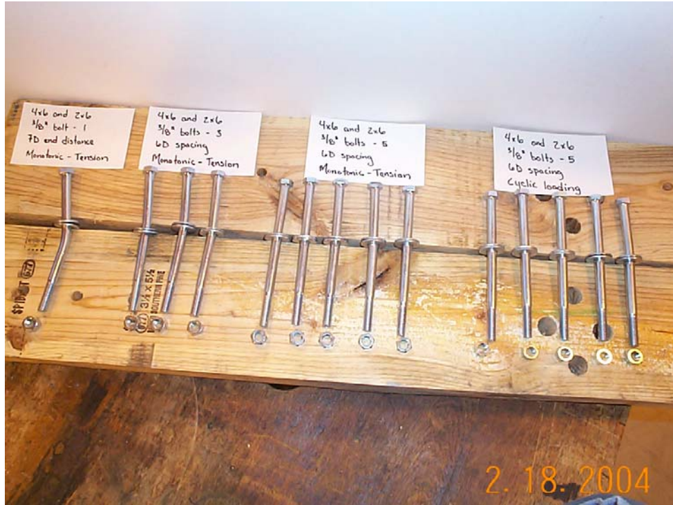
Figure 4.32: Bolts from Alternate Connection Configurations.
