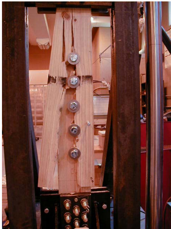
Figure 4.3: Typical Expected Yield Mode II Connection under Cyclic Loading, 5D spacing.
