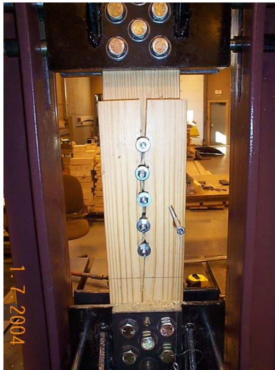
Figure 4.9: Typical Expected Yield Mode IV Connection under Cyclic Loading, 5D spacing.
