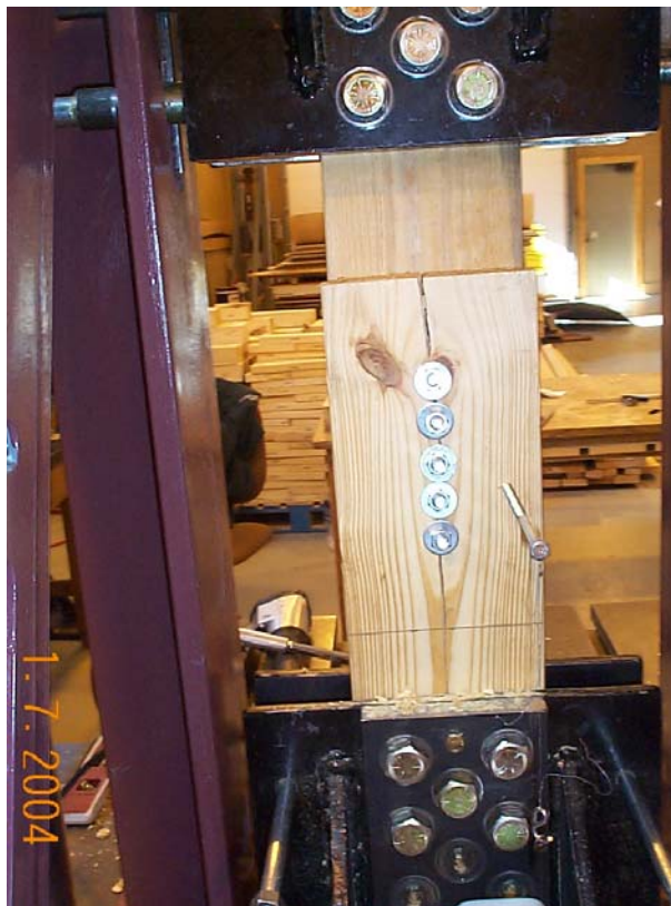
Figure 4.8: Typical Expected Yield Mode IV Connection under Monotonic Loading, 3D spacing.
