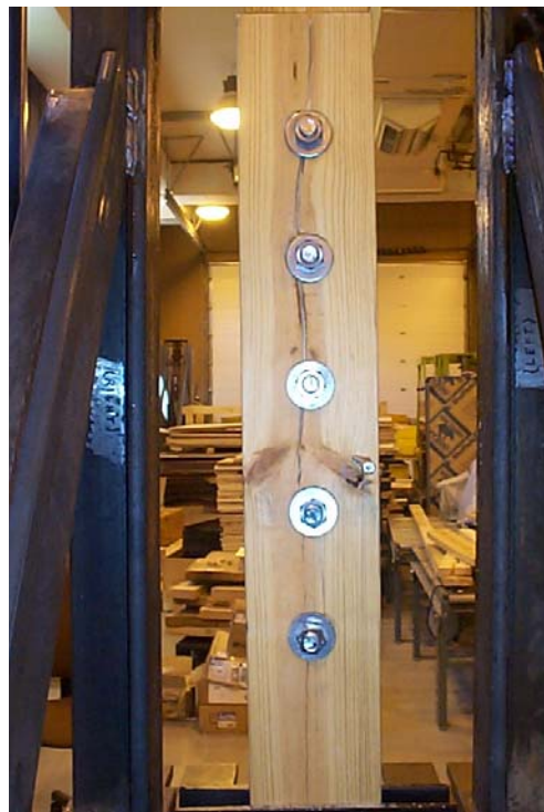
Figure 4.2: Typical Expected Yield Mode II Connection under Monotonic Loading, 7D spacing.
