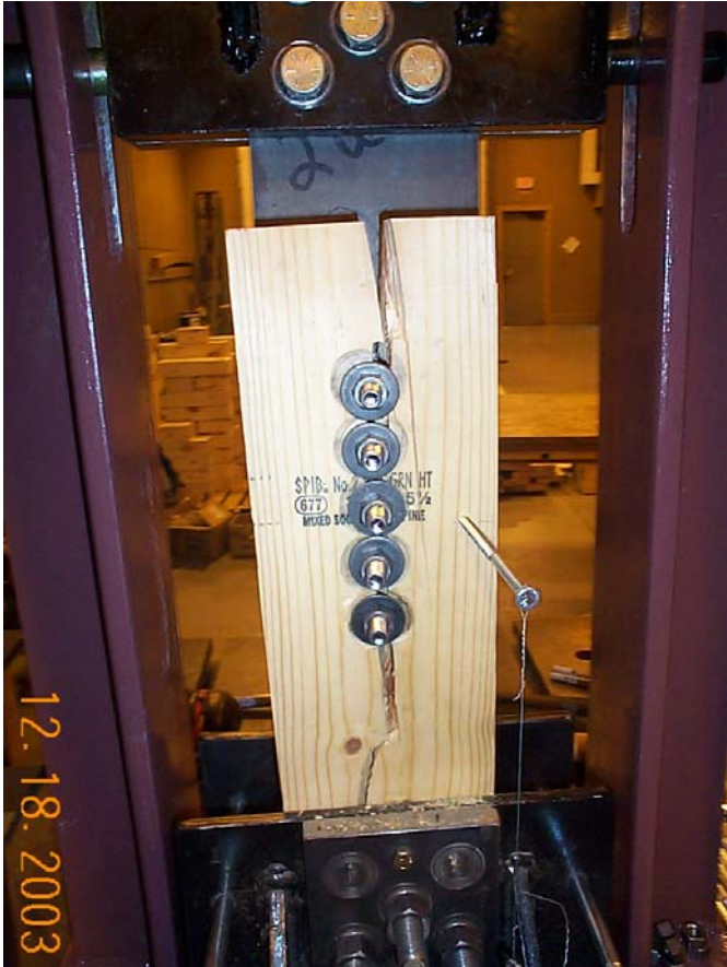
Figure 4.6: Typical Expected Yield Mode III Connection under Cyclic Loading, 3D spacing.
