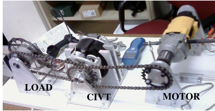
Figure 6-13. The current dynamometer setup including the current CIVT design. The three components of the design are connected together by a chain.
