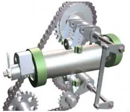
Figure 5-1. Model of Naude's cam driven IVT with cylindrical rollers [33].
