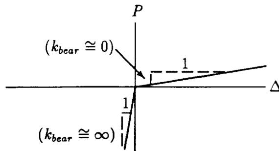
Figure 3.5: Load Displacement Relationship for Bearing Element (White, 1995)
