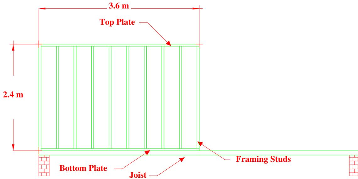
Figure 3.12: Shear Wall Model on a Flexible Foundation
