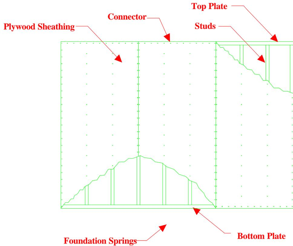
Figure 3.11: 2.4 m x 3.7 m Shear Wall Model
