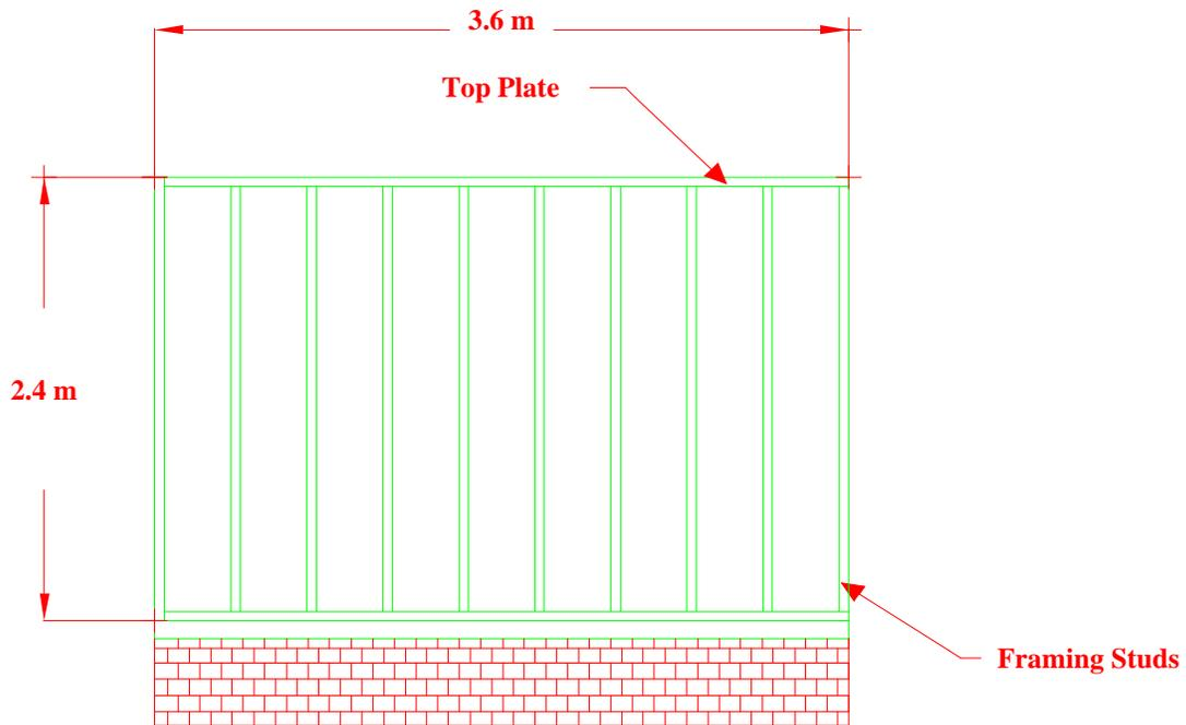
Figure 3.13: Shear Wall Model on a Rigid Foundation
