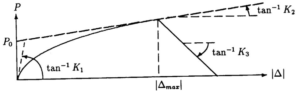
Figure 3.3: Load Displacement Curve for the Connector Elements Subjected to Monotonic Loading (Dolan, 1989)
