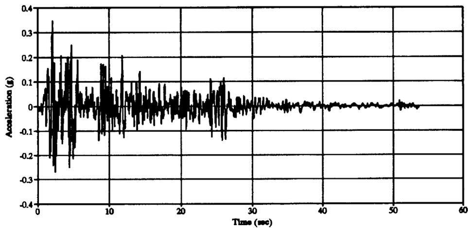
Figure 3.16: Acceleration Record for the S00E Component of the 1940 El Centro Earthquake (White, 1995)
