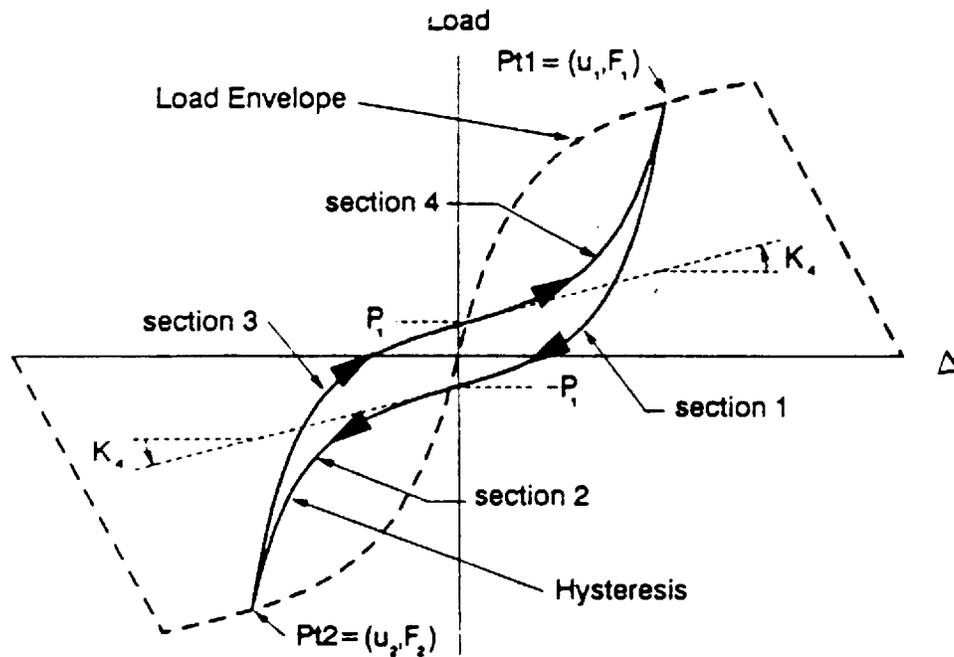
Figure 3.4: Load Displacement Curve for the Connector Elements Subjected to Dynamic Loading (Dolan, 1989)
