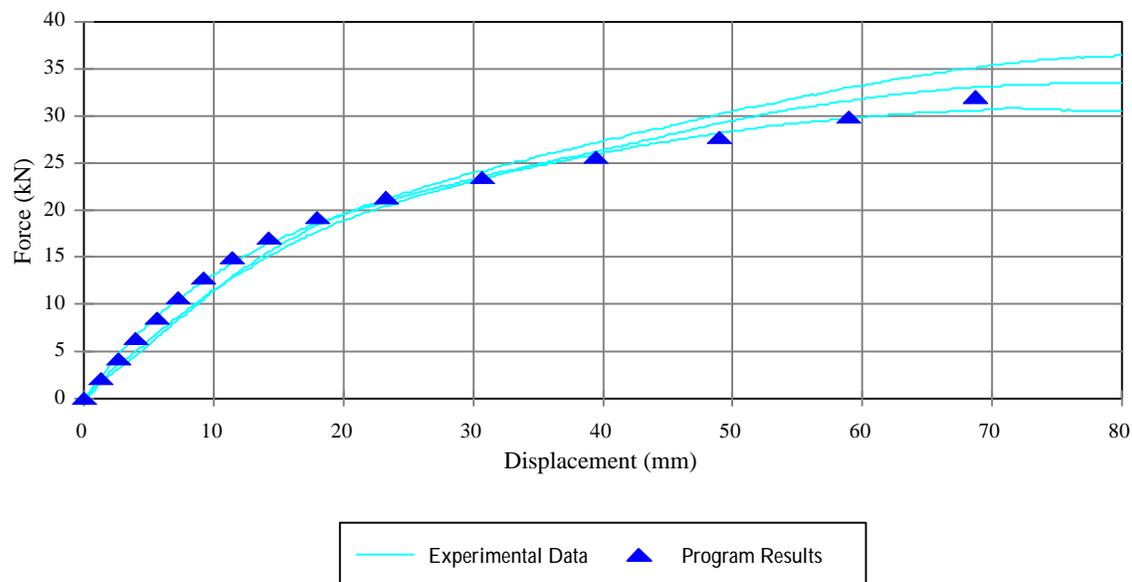
Figure 3.9: Monotonic Load-Displacement Curve from Validation Test for WALSEIZ1
