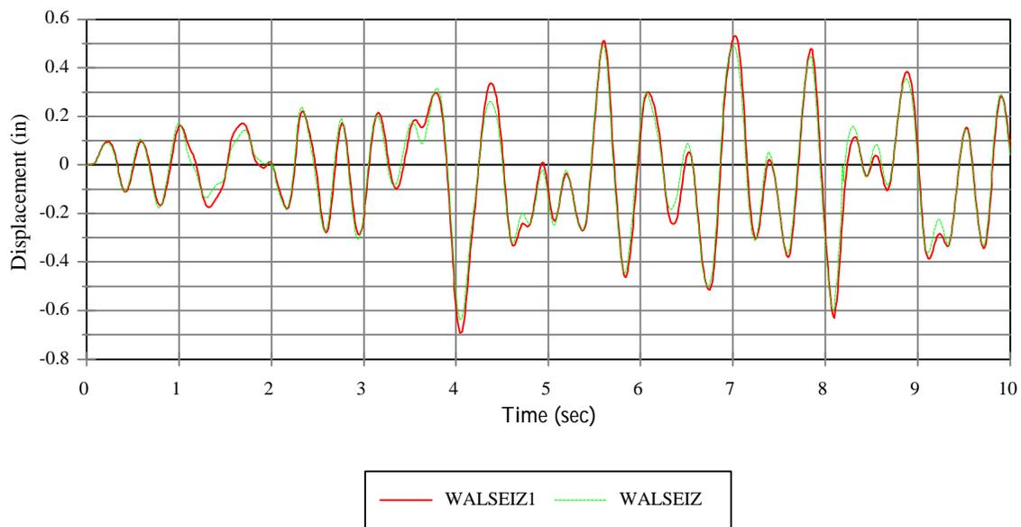
Figure 3.10: Dynamic Time-Displacement Curve from Validation Test for WALSEIZ1
