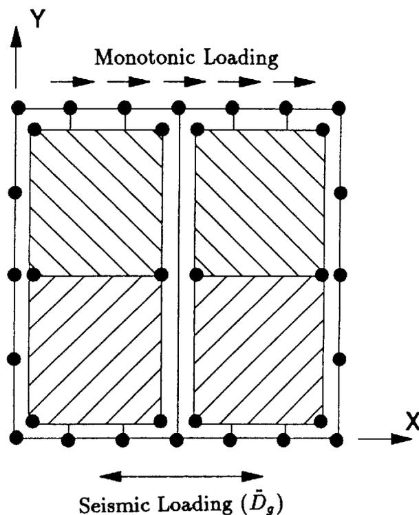
Figure 3.8: Loading Applied to Shear Wall Model (White, 1995)
