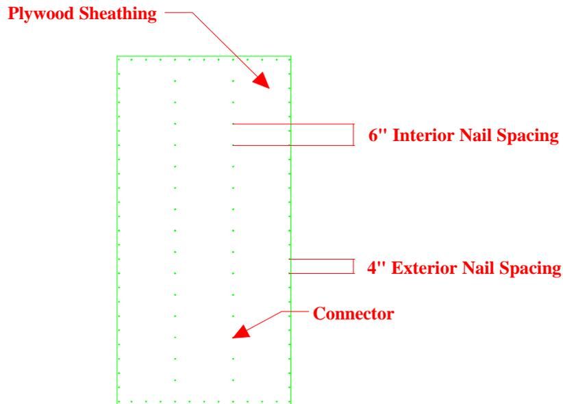
Figure 3.15: Nail Spacing for a Typical Sheathing Panel
