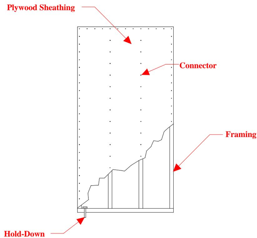
Figure 1.1: Components of a Typical Shear Wall
