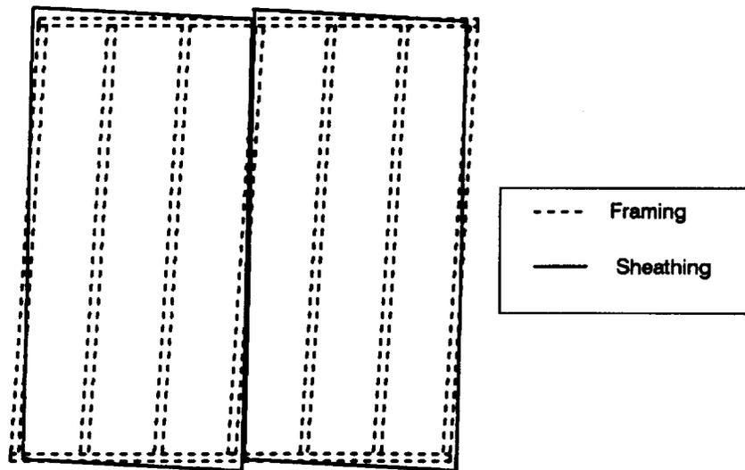
Figure 2.1: Deformation Pattern of a Shear Wall (White, 1995)
