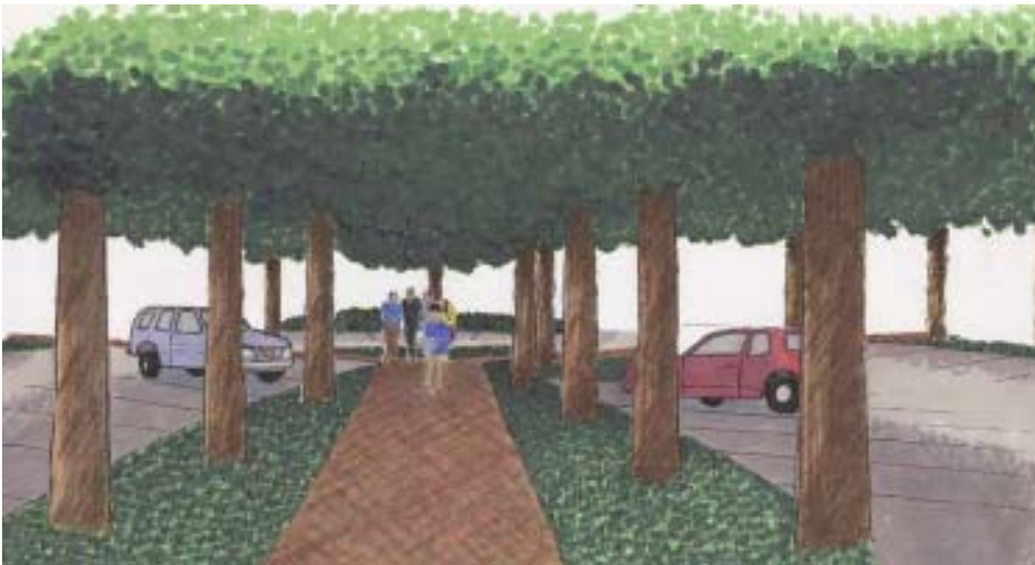
Figure 6.7. Design One Perspective. Clustered trees provide plenty of shade for the parking lot as well as bringing the scale of the lot to the pedestrian level.
