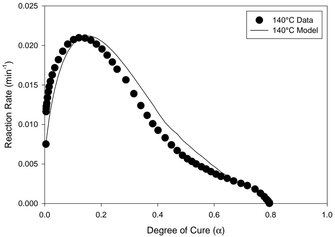
**Figure 3.37: Comparison between experimental and model values for reaction rate as a function of degree of cure for 140°C.**
