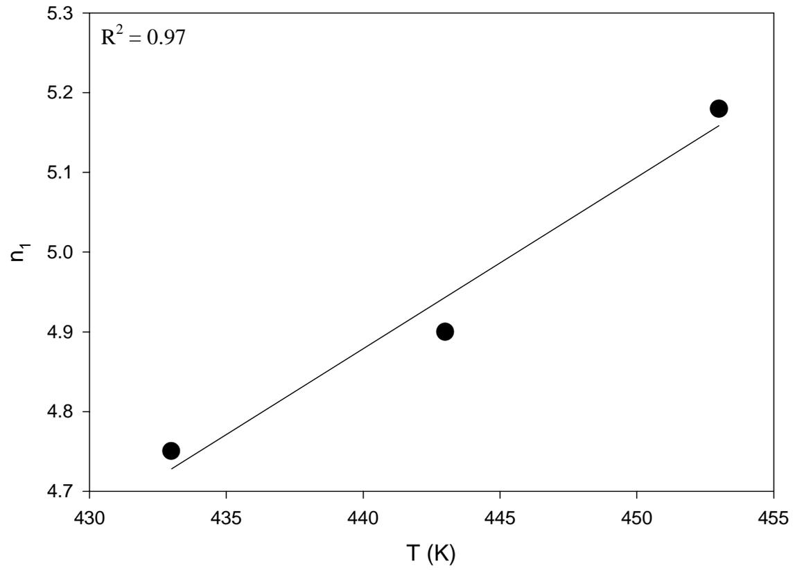
**Figure 3.24: Kinetic exponent,  $n_1$ , as a function of temperature between 160 and 180°C for Fiberite 954-2a resin.**
