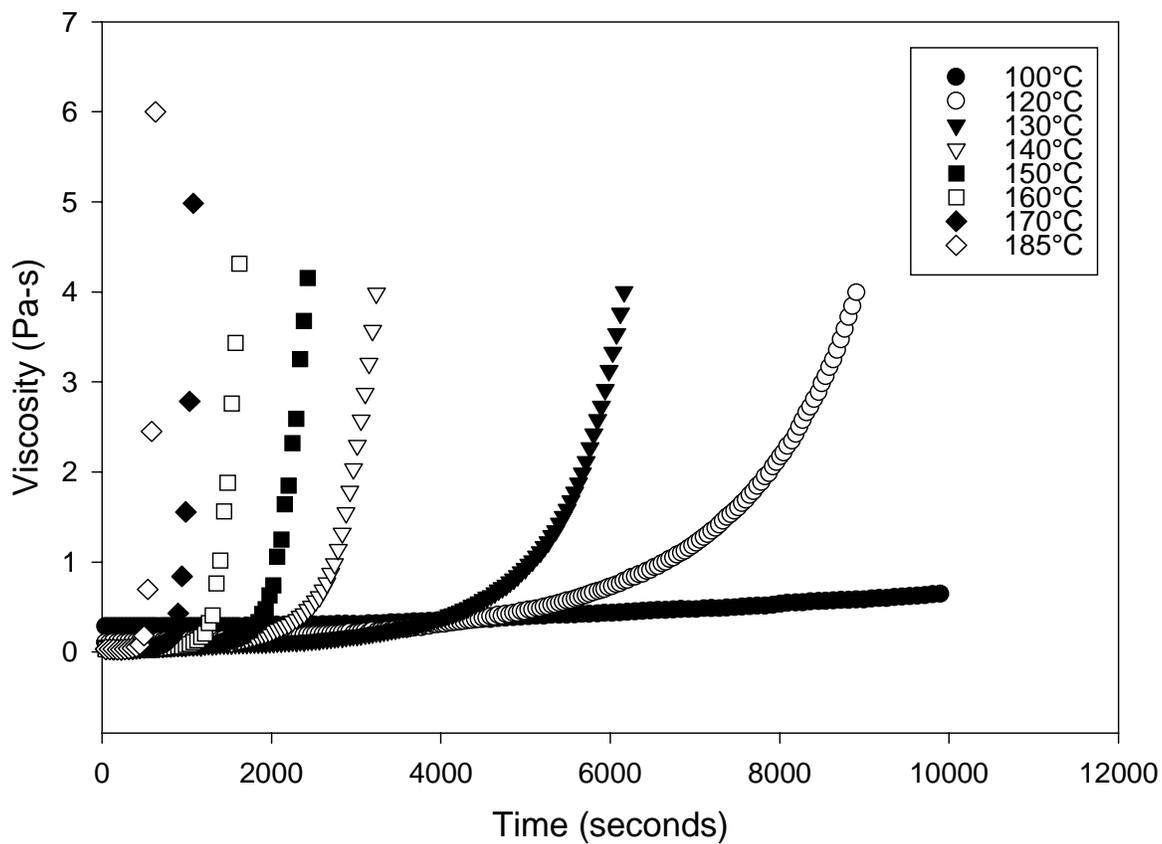
**Figure 4.1: Measured viscosity as a function of time at different isothermal temperatures for the 954-3 cyanate ester resin system.**
