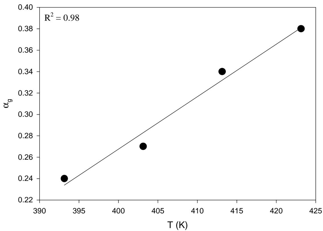
**Figure 4.12: Temperature dependence of the degree of cure at gel for 954-2a.**
