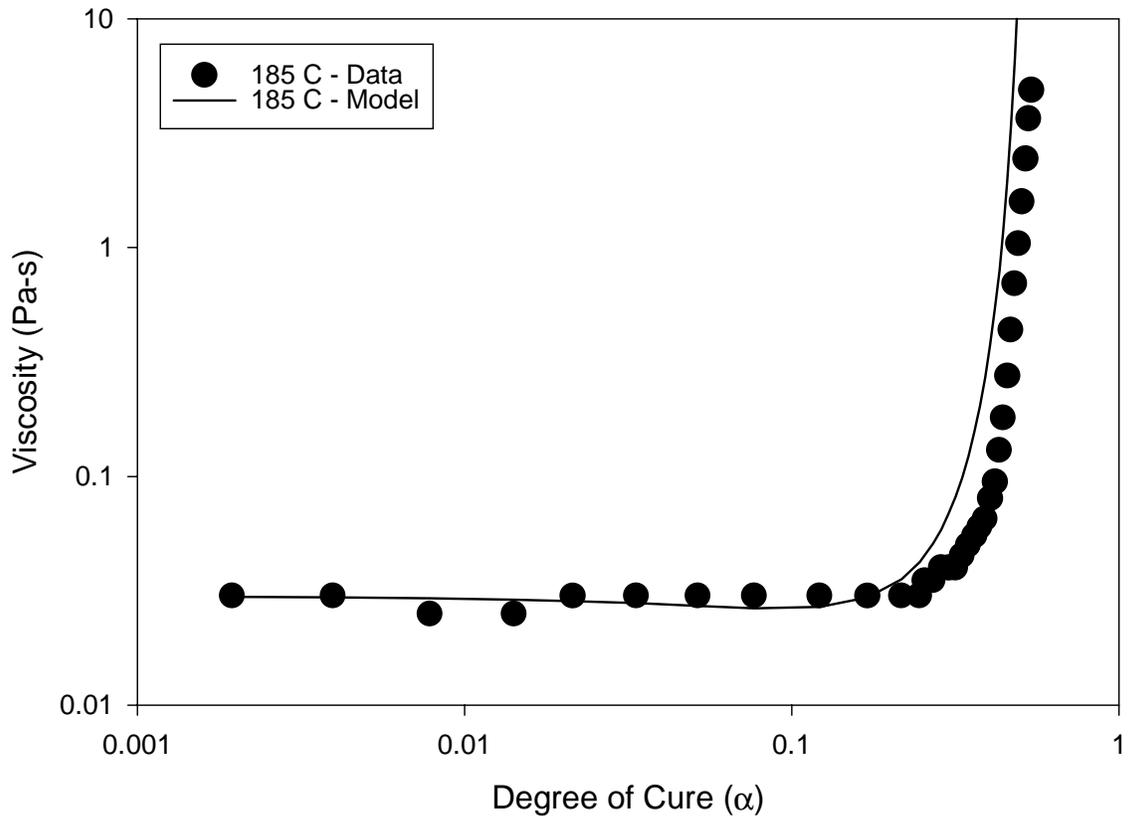
**Figure 4.9: Comparison of measured and model predicted viscosity as a function of time at 185°C for 954-3 cyanate ester resin.**
