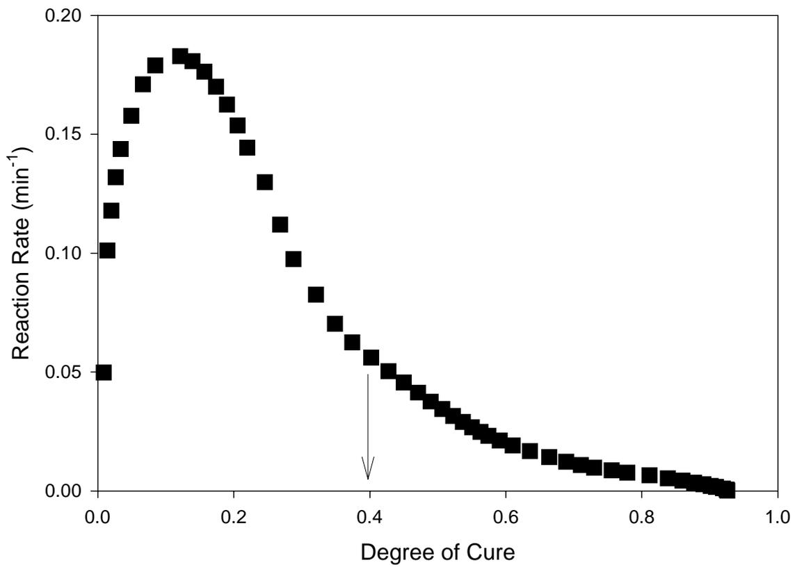
**Figure 3.5: Plot of reaction rate vs. degree of cure for 954-2a, run at 180°C, showing the determination of  $\alpha_d$ .**
