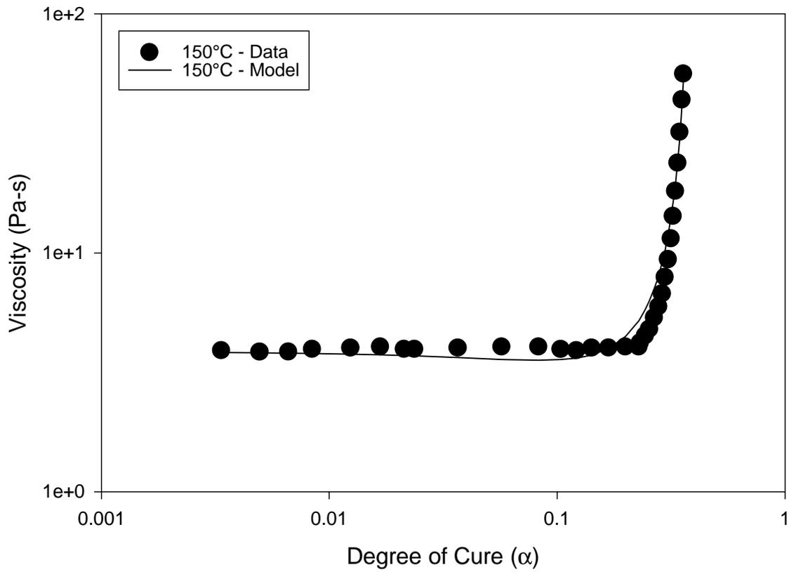
**Figure 4.18: Comparison of measured and model predicted viscosity as a function of time at 150°C for 954-2a toughened cyanate ester resin.**
