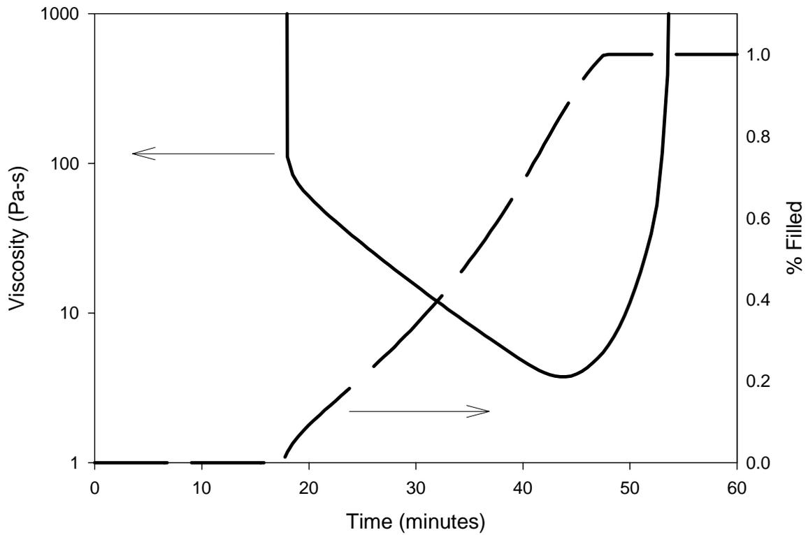
**Figure 6.5: Viscosity and resin infiltration as a function of time for the 954-2a cyanate ester resin flowing through the EWC-600X 8HS graphite fabric.**
