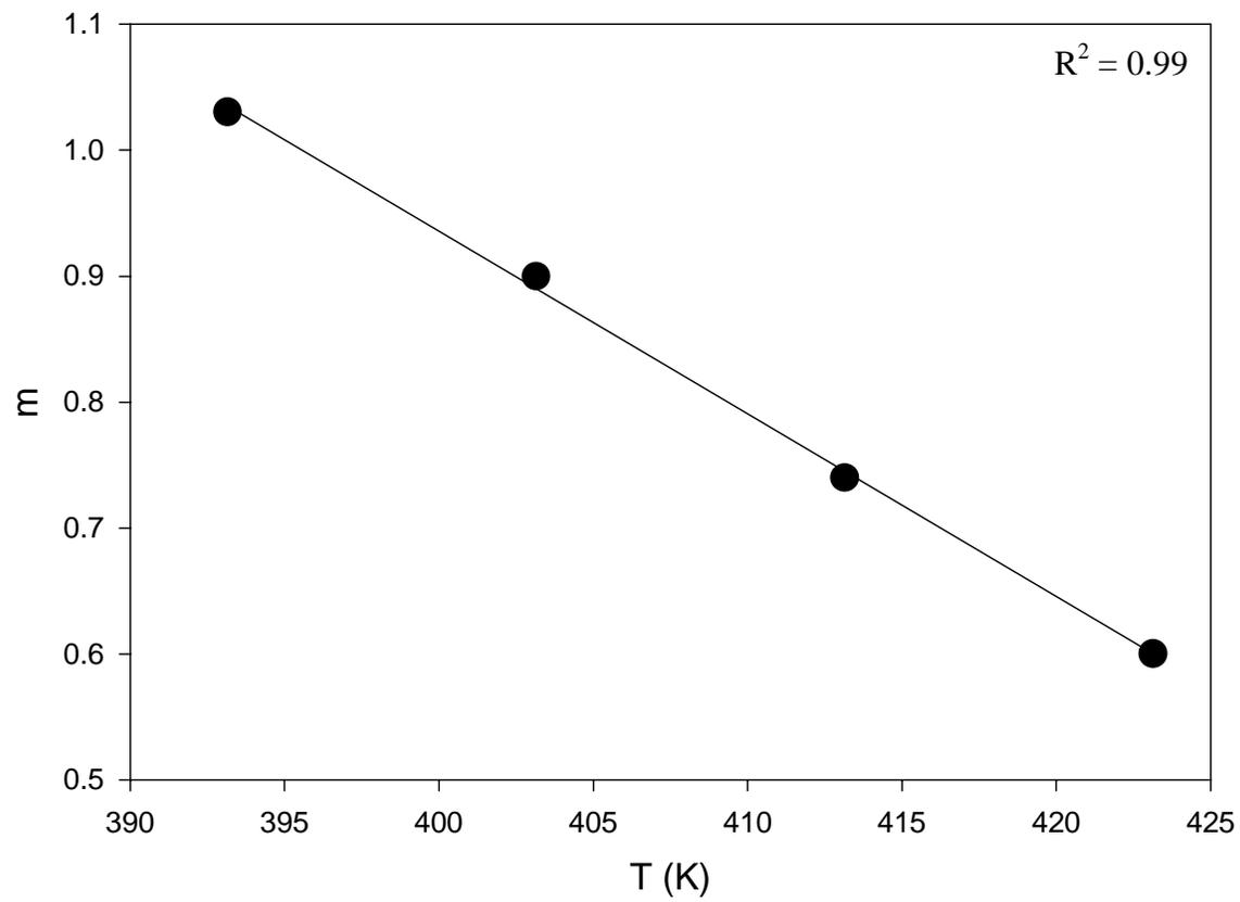
**Figure 3.29: Kinetic exponent,  $m$ , as a function of temperature between 120 and 160°C for Fiberite 954-2a resin.**
