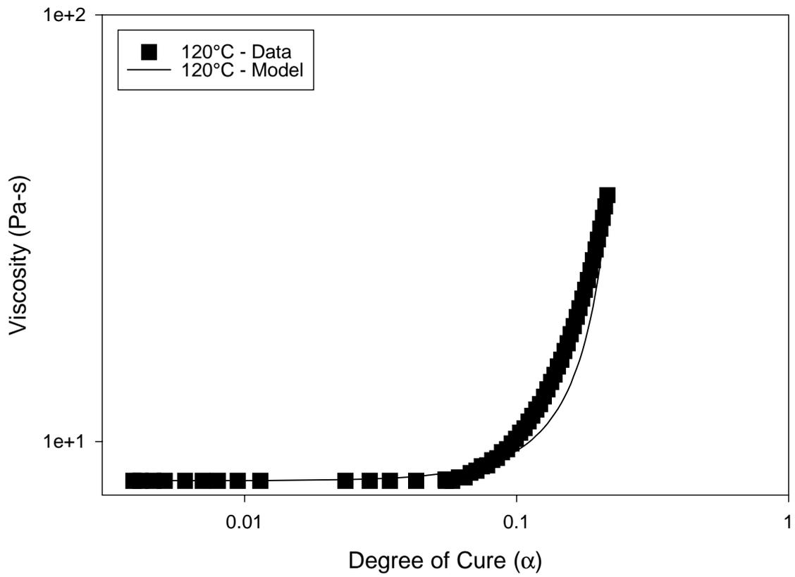
**Figure 4.15: Comparison of measured and model predicted viscosity as a function of time at 120°C for 954-2a toughened cyanate ester resin.**
