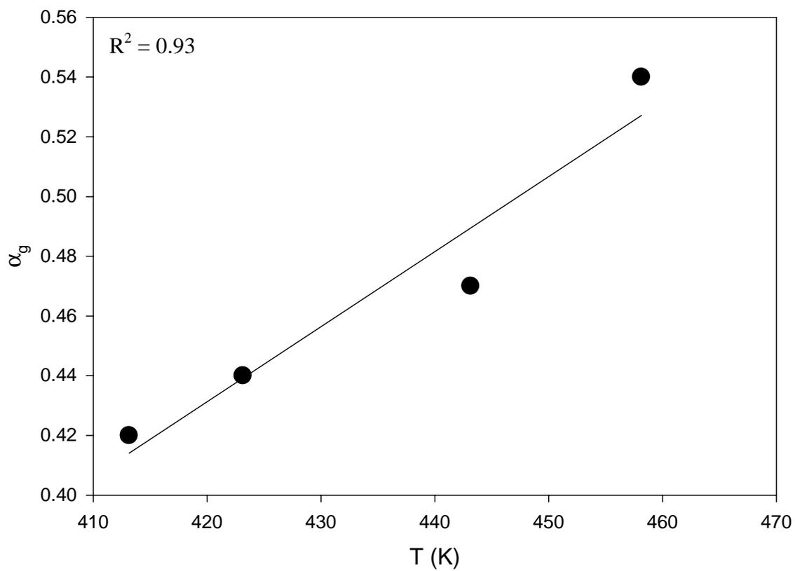
**Figure 4.3: Temperature dependence of the degree of cure at gel for 954-3.**
