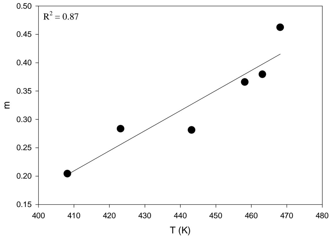
**Figure 3.10: Kinetic exponent,  $m$ , as a function of temperature for Fiberite 954-3 resin.**
