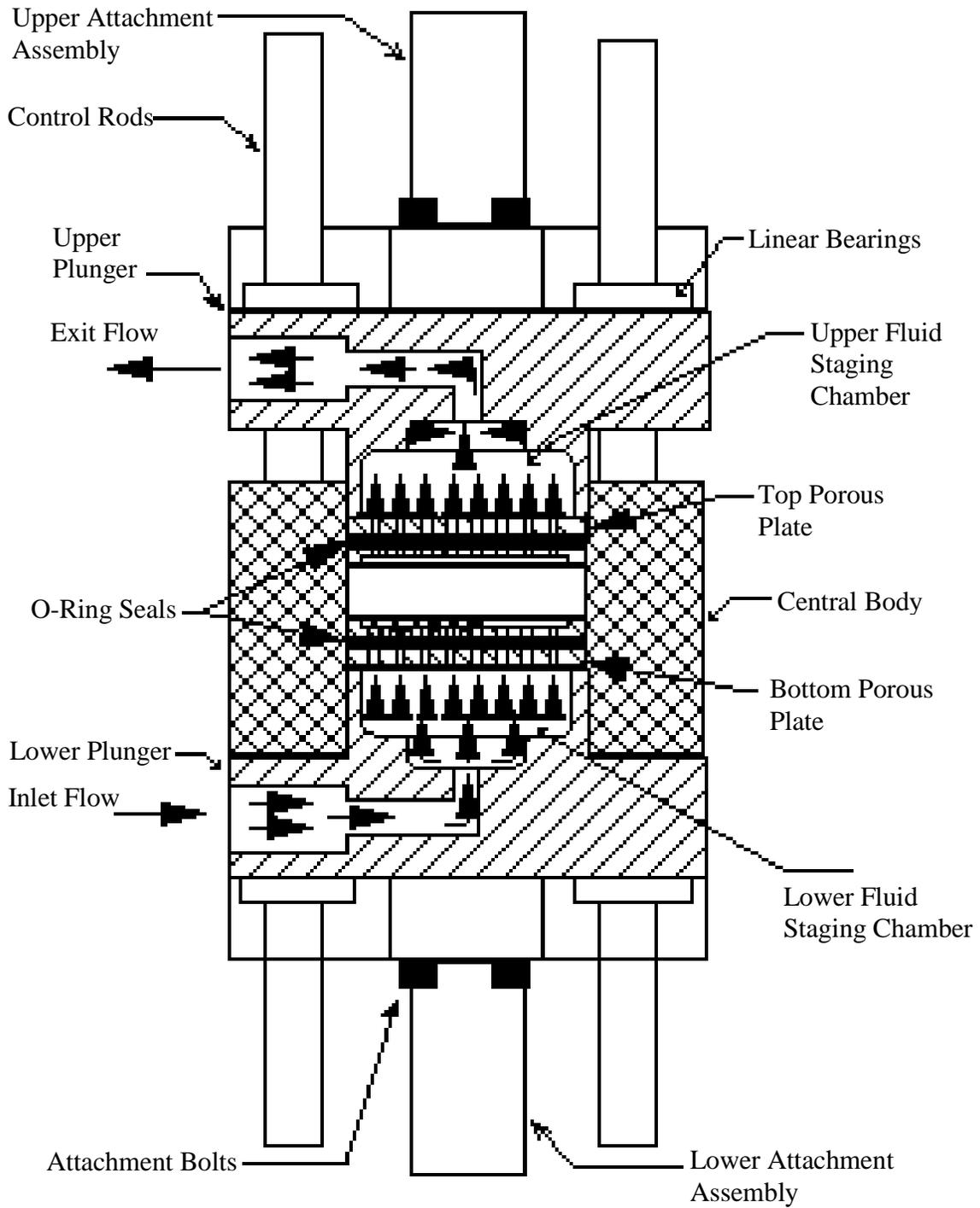
**Figure 5.1: Schematic of the 5.08 cm x 5.08 cm through the thickness permeability fixture [35].**
