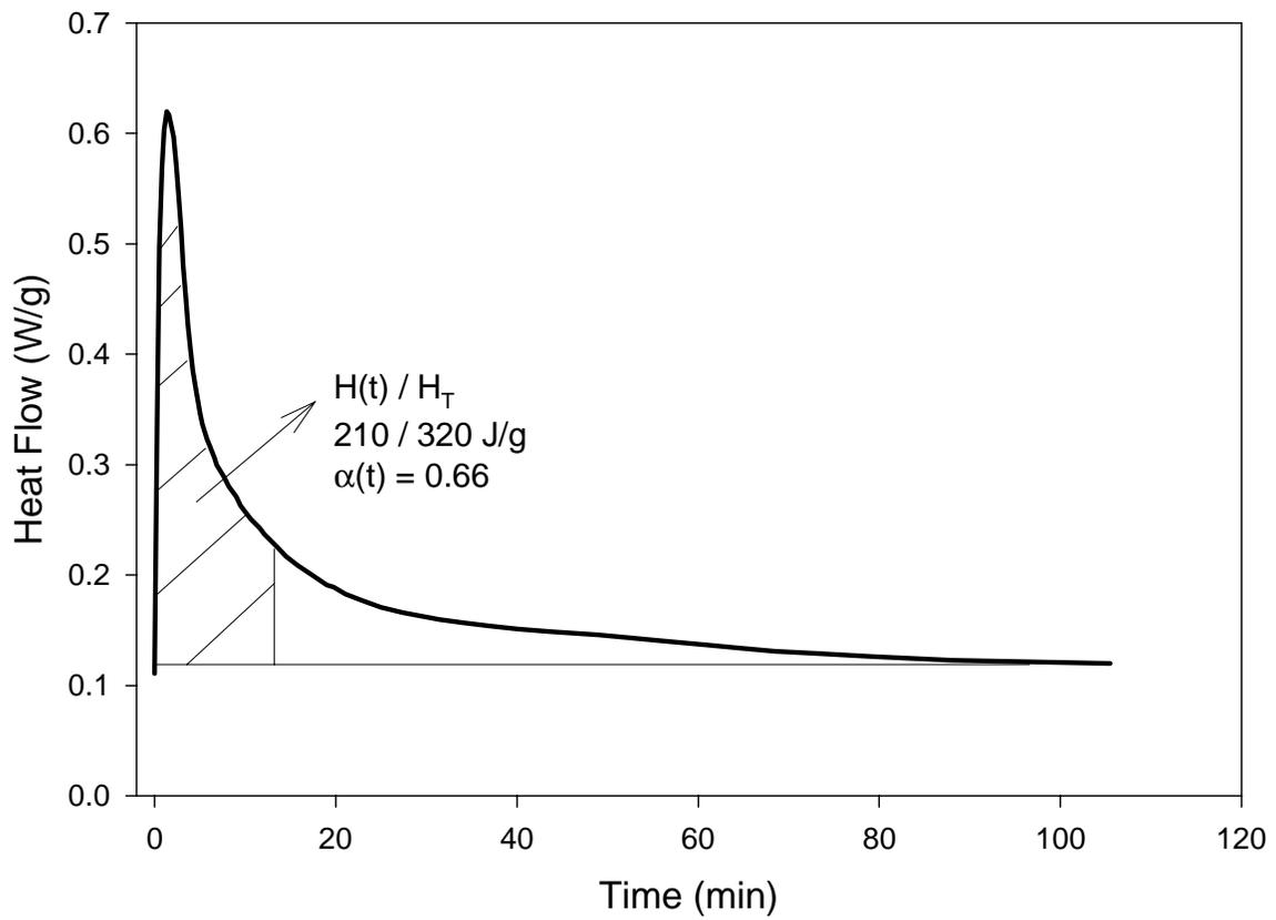
**Figure 3.4:** Example of an isothermal scan broken up into intervals to determine the degree of cure as a function of time.
