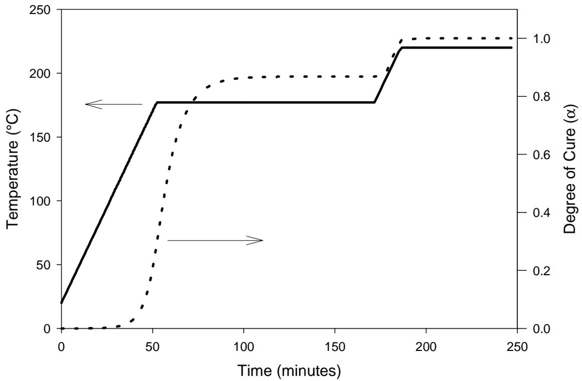
**Figure 6.6: Temperature and degree of cure as a function of time for the 954-3 cyanate ester resin flowing through the TTI IM7/ 8HS carbon fabric.**
