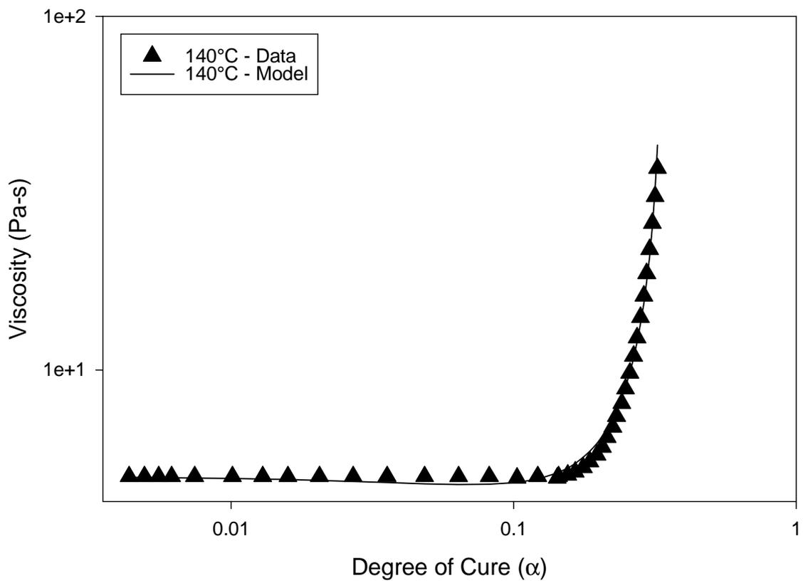
**Figure 4.17: Comparison of measured and model predicted viscosity as a function of time at 140°C for 954-2a toughened cyanate ester resin.**
