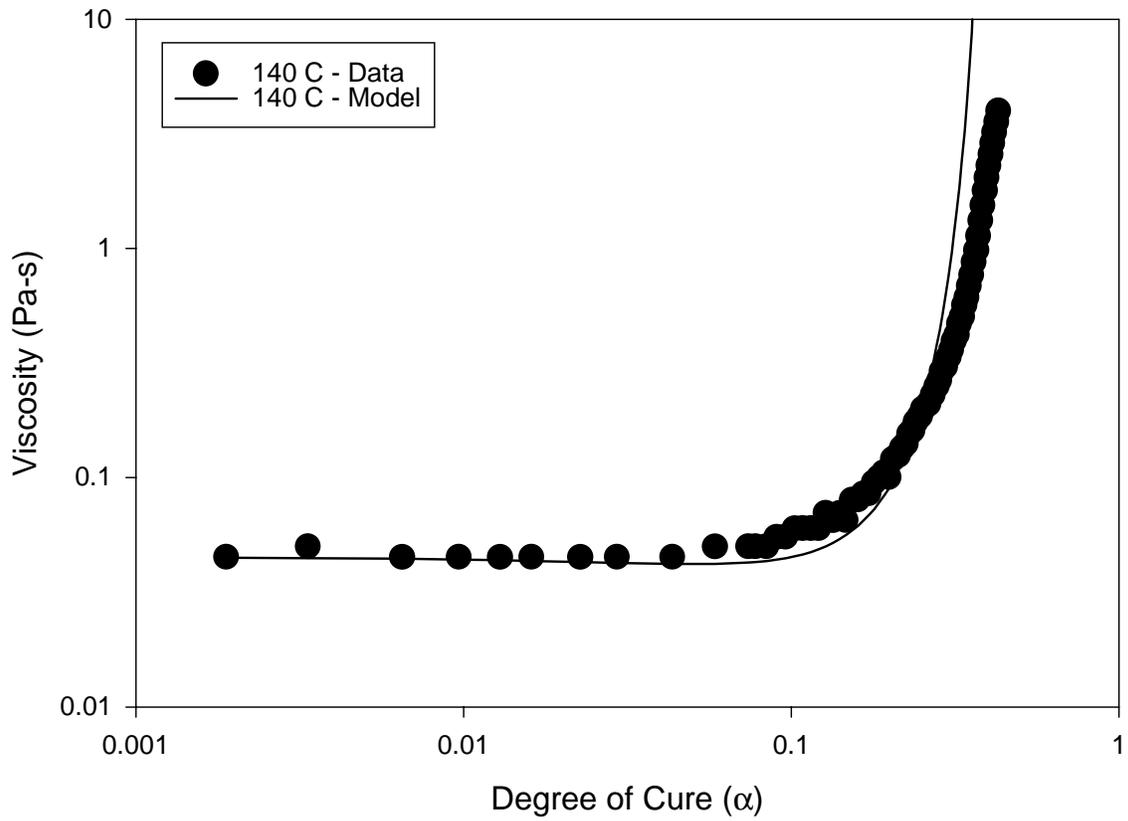
**Figure 4.6: Comparison of measured and model predicted viscosity as a function of time at 140°C for 954-3 cyanate ester resin.**
