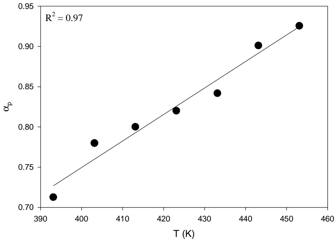
**Figure 3.32: Plot of peak degree of cure vs. temperature for Fiberite 954-2a resin.**
