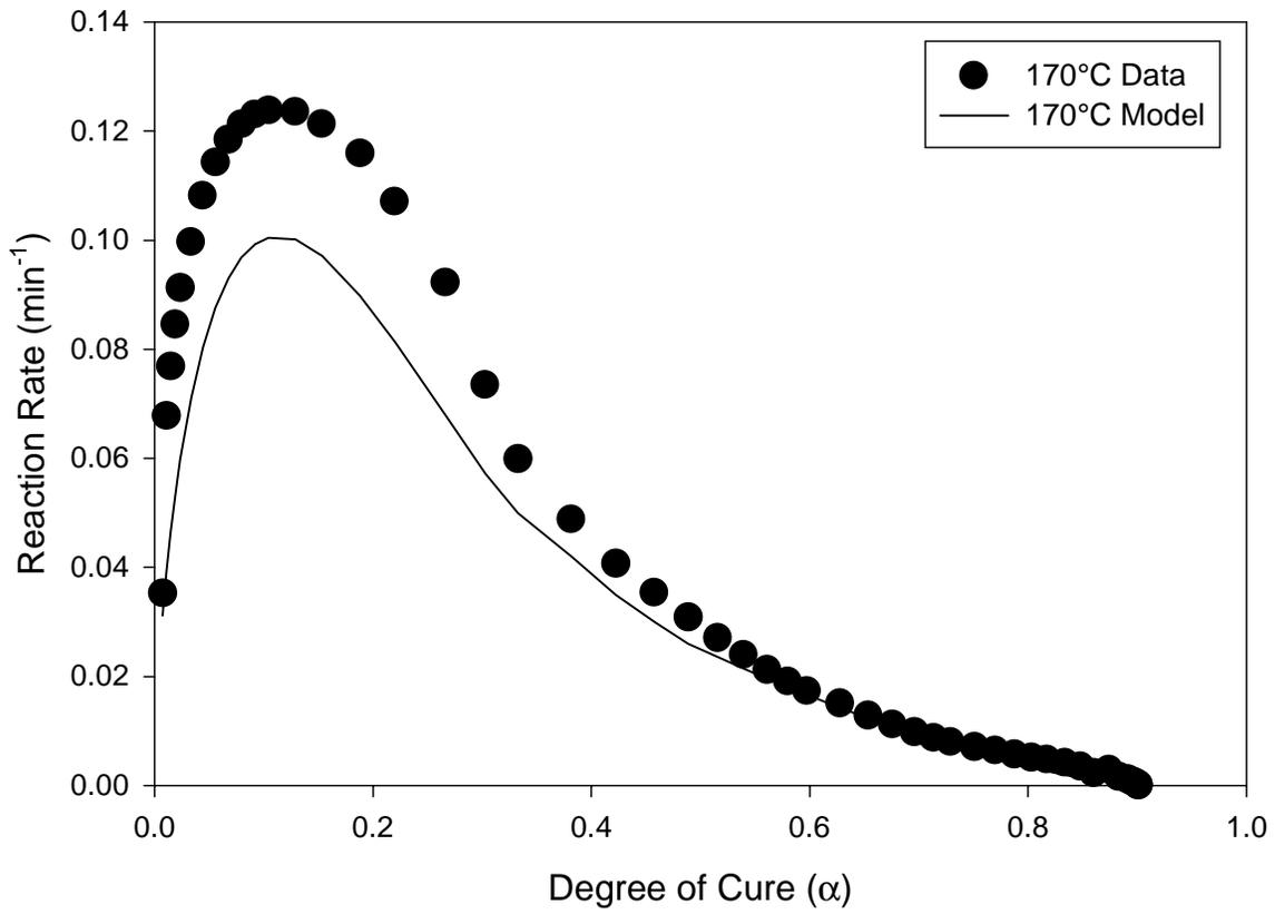
**Figure 3.34: Comparison between experimental and model values for reaction rate as a function of degree of cure for 170°C.**
