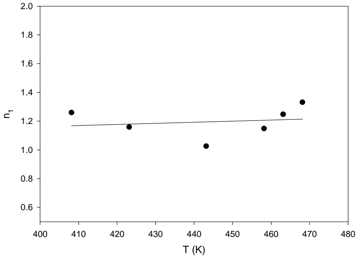
**Figure 3.11: Kinetic exponent,  $n_1$ , as a function of temperature for Fiberite 954-3 resin.**
