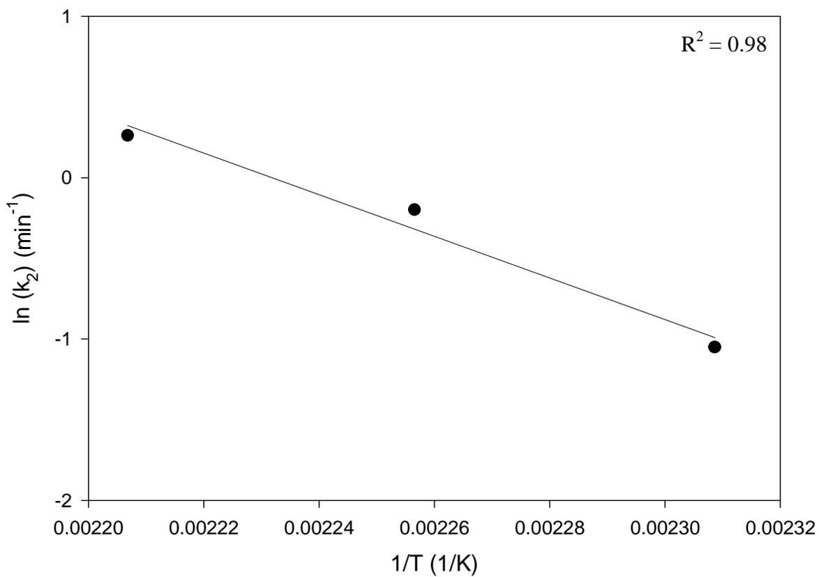
**Figure 3.21: Plot of  $\ln(k_2)$  vs.  $1/T$  for temperatures between 160 and 180°C for Fiberite 954-2a resin.**
