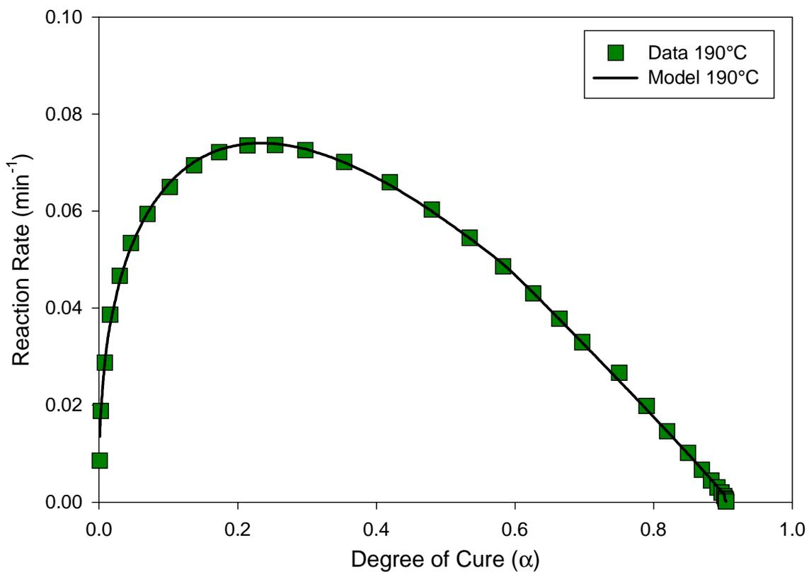
**Figure 3.15: Comparison between experimental and model values for reaction rate as a function of degree of cure for  $190^{\circ}\text{C}$ .**
