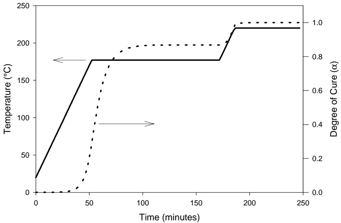
**Figure 6.2: Temperature and degree of cure as a function of time for the 954-3 cyanate ester resin flowing through the EWC-600X 8HS graphite fabric.**
