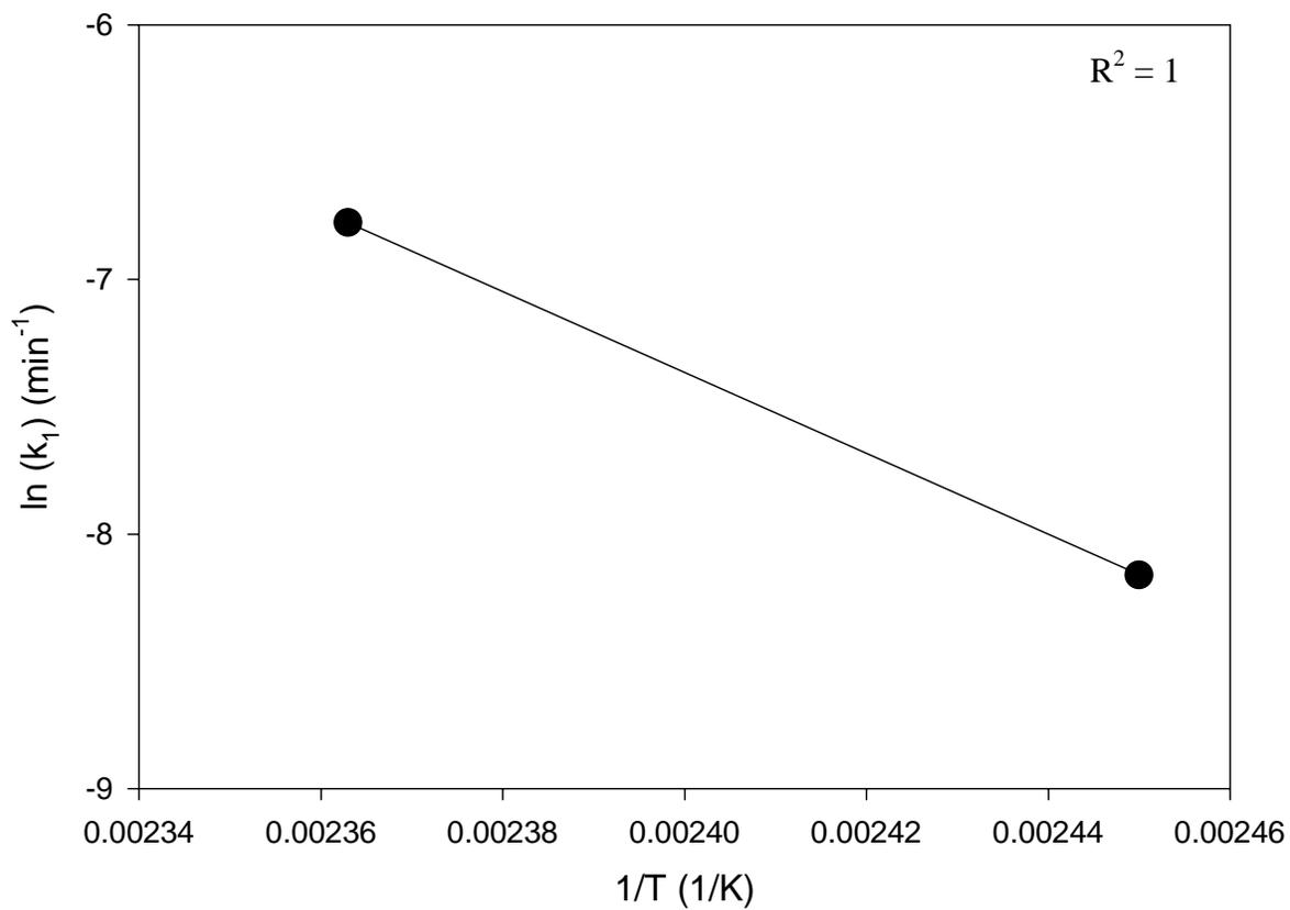
**Figure 3.7: Plot of  $\ln(k_1)$  vs.  $1/T$  for temperatures between 135°C and 150°C for Fiberite 954-3 resin.**
