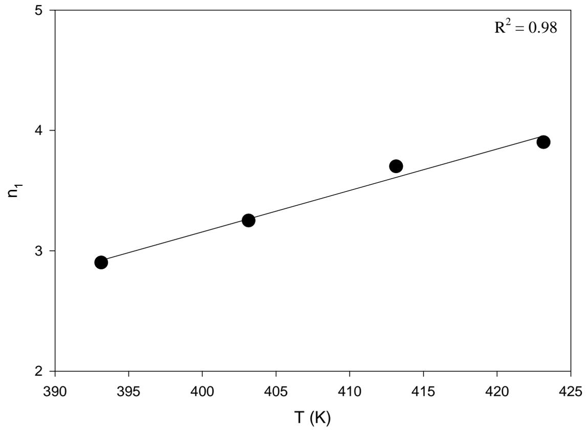
**Figure 3.30: Kinetic exponent,  $n_1$ , as a function of temperature between 120 and 160°C for Fiberite 954-2a resin.**
