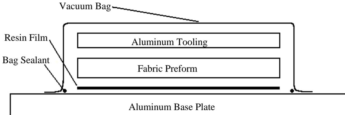
**Figure 6.1: Exploded view of the Resin Film Infusion Setup.**
