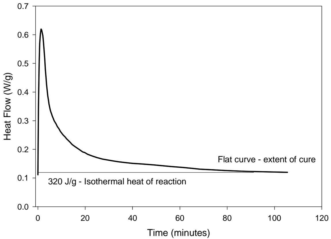
**Figure 3.2: Example isothermal scan, run at 180°C for 110 minutes on the 954-2a resin, showing the isothermal heat of reaction ( $H_{iso}$ ).**
