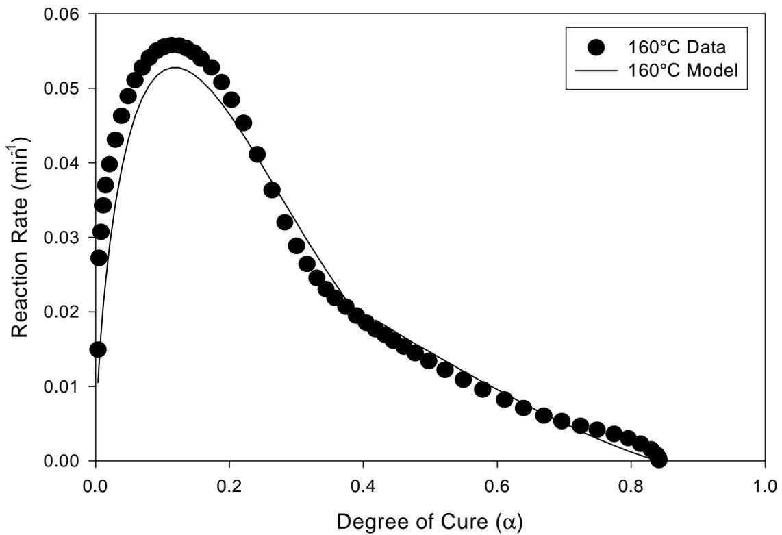
**Figure 3.35: Comparison between experimental and model values for reaction rate as a function of degree of cure for 160°C.**
