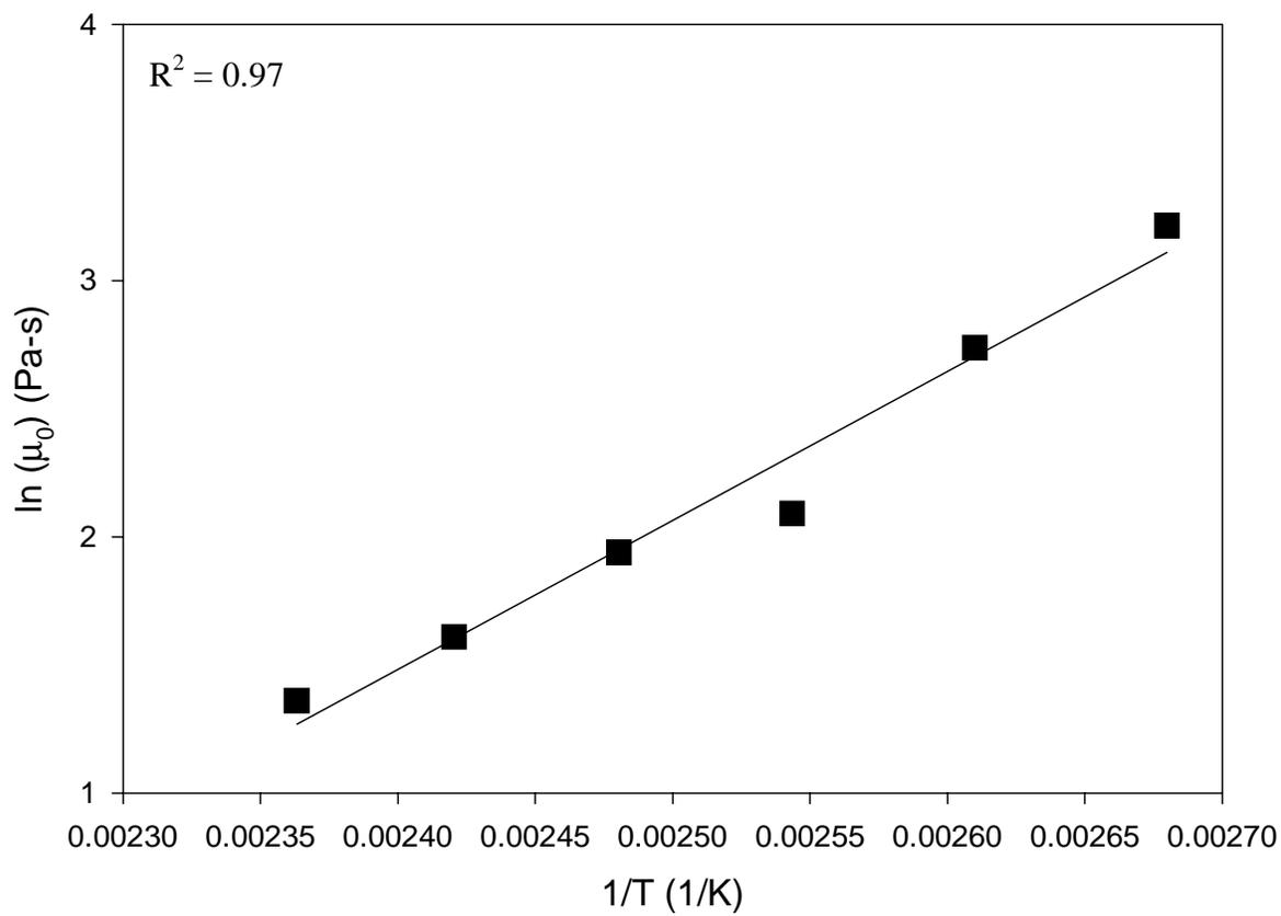
**Figure 4.11: Arrhenius plot showing the temperature dependence of initial viscosity for 954-2a.**
