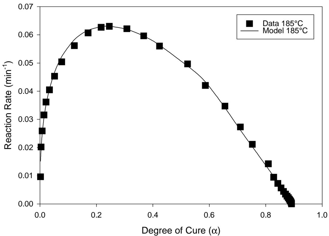
**Figure 3.16: Comparison between experimental and model values for reaction rate as a function of degree of cure for 185°C.**
