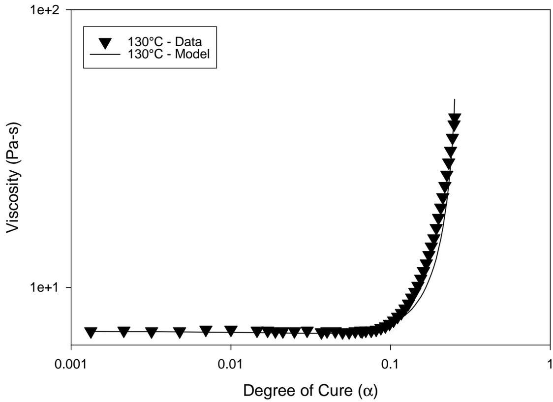
**Figure 4.16: Comparison of measured and model predicted viscosity as a function of time at 130°C for 954-2a toughened cyanate ester resin.**
