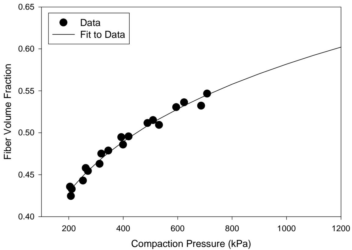
**Figure 5.2: Fiber volume fraction as a function of applied compaction pressure for Amoco Thermalgraph™ EWC-600X 8HS graphite fabric.**
