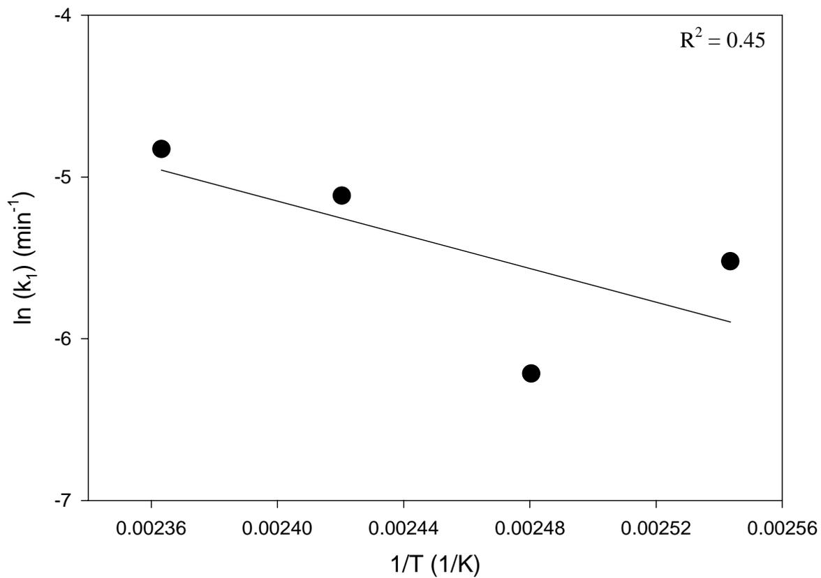
**Figure 3.26: Plot of  $\ln(k_1)$  vs.  $1/T$  for temperatures between 120 and 160°C for Fiberite 954-2a resin.**
