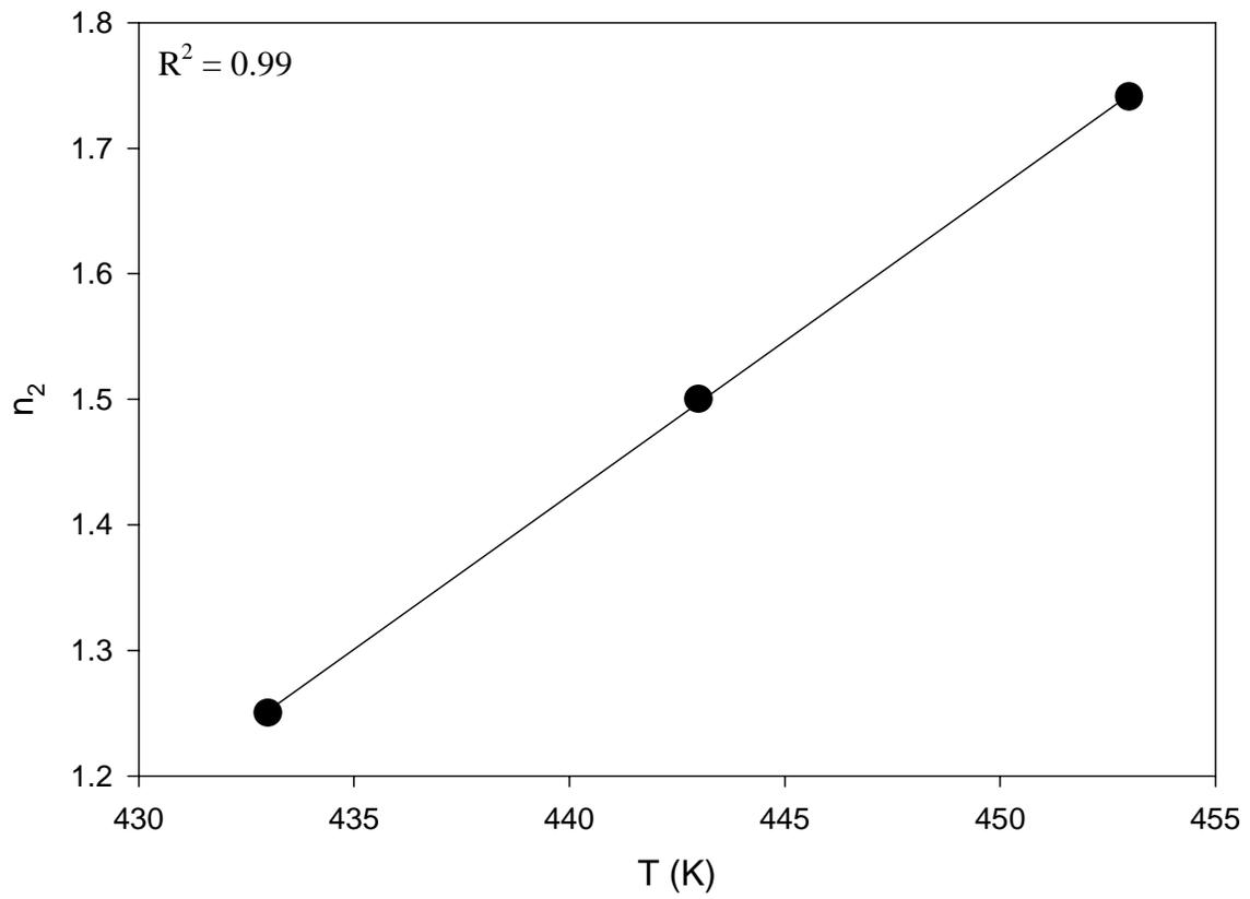
**Figure 3.25: Kinetic exponent,  $n_2$ , as a function of temperature between 160 and 180°C for Fiberite 954-2a resin.**
