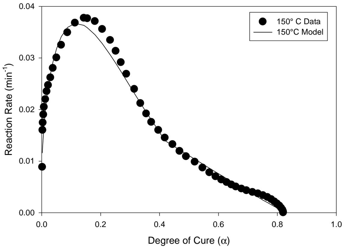
**Figure 3.36: Comparison between experimental and model values for reaction rate as a function of degree of cure for 150°C.**
