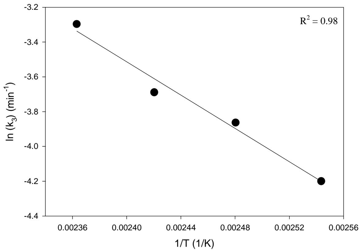
**Figure 3.28: Plot of  $\ln(k_3)$  vs.  $1/T$  for temperatures between 120 and 160°C for Fiberite 954-2a resin.**
