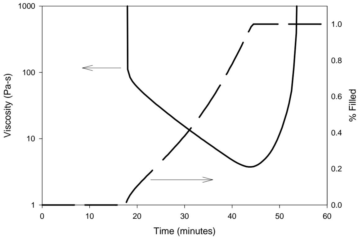
**Figure 6.9: Viscosity and resin infiltration as a function of time for the 954-2a cyanate ester resin flowing through the TTI IM7/ 8HS carbon fabric.**
