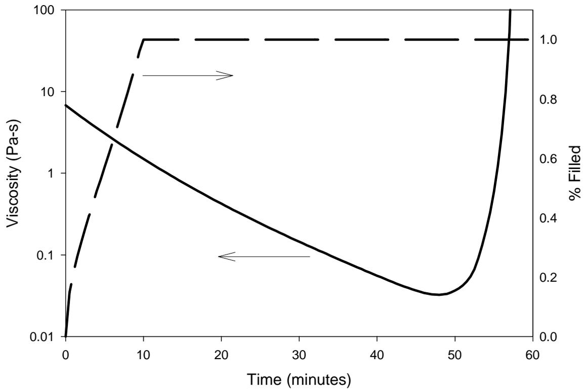
**Figure 6.3: Viscosity and resin infiltration as a function of time for the 954-3 cyanate ester resin flowing through the EWC-600X 8HS graphite fabric.**
