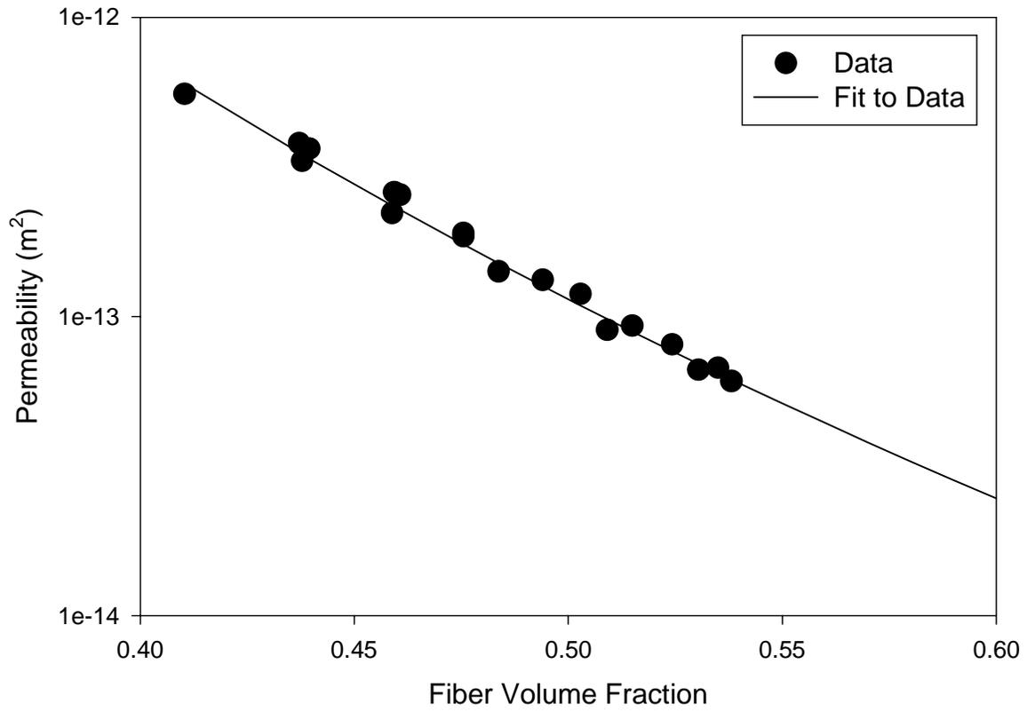
**Figure 5.3: Permeability behavior for the EWC-600X 8HS graphite fabric in the through-the-thickness direction.**
