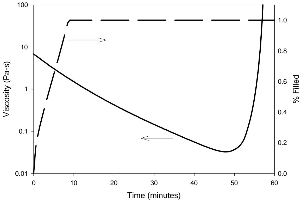
**Figure 6.7: Viscosity and resin infiltration as a function of time for the 954-3 cyanate ester resin flowing through the TTI IM7/ 8HS carbon fabric.**
