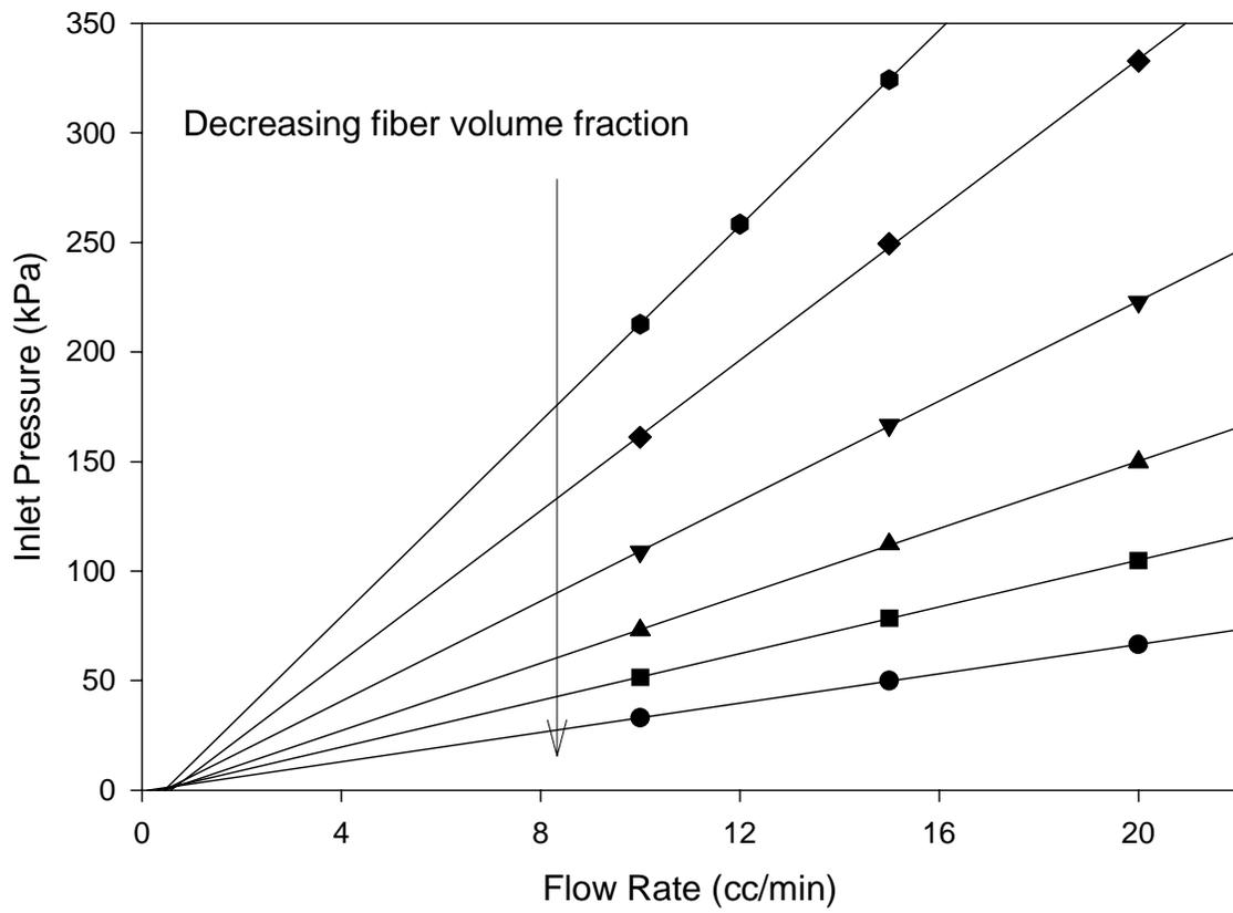
**Figure 5.4: Inlet pressure as a function of flow rate for EWC-600X 8HS graphite fabric.**
