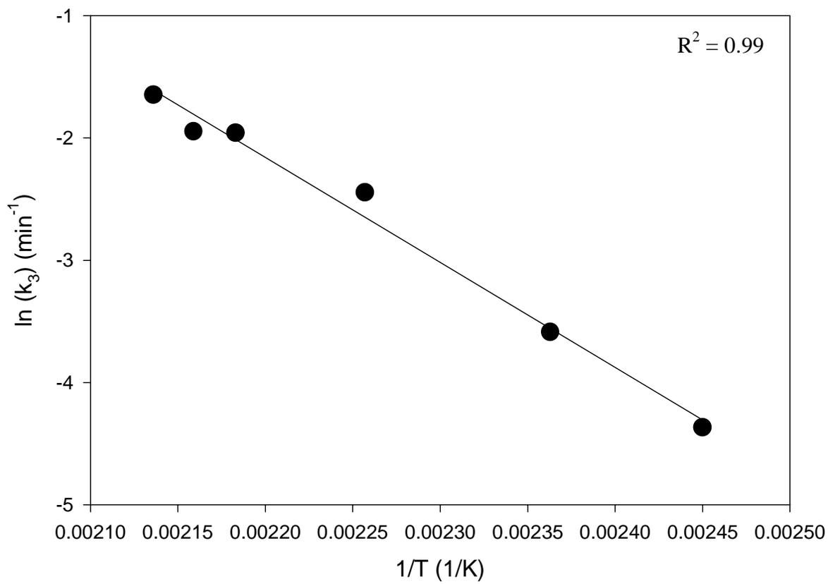
**Figure 3.9: Plot of  $\ln(k_3)$  vs.  $1/T$  for Fiberite 954-3 resin.**
