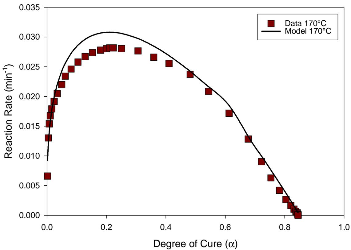
**Figure 3.17: Comparison between experimental and model values for reaction rate as a function of degree of cure for 170°C.**
