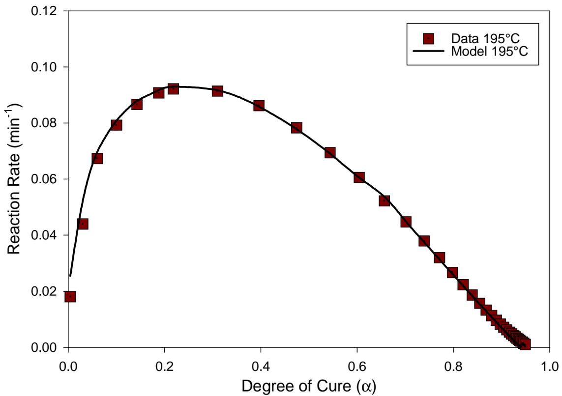
**Figure 3.14: Comparison between experimental and model values for reaction rate as a function of degree of cure for 195°C.**
