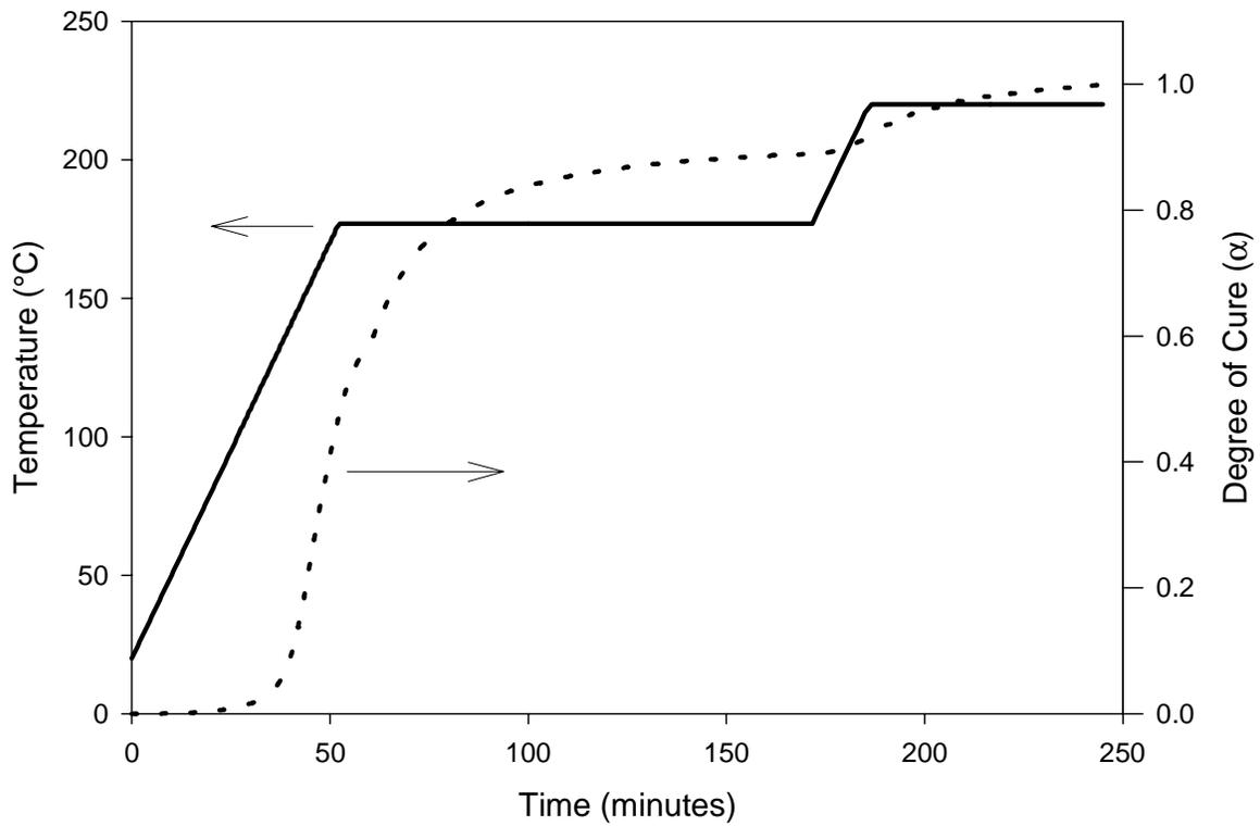
**Figure 6.8: Temperature and degree of cure as a function of time for the 954-2a cyanate ester resin flowing through the TTI IM7/ 8HS carbon fabric.**
