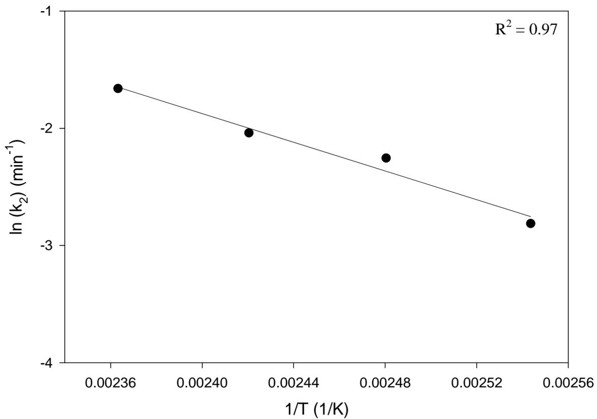
**Figure 3.27: Plot of  $\ln(k_2)$  vs.  $1/T$  for temperatures between 120 and 160°C for Fiberite 954-2a resin.**
