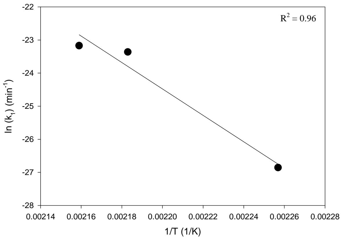
**Figure 3.6: Plot of  $\ln(k_1)$  vs.  $1/T$  for temperatures between 170°C and 195°C for Fiberite 954-3 resin.**
