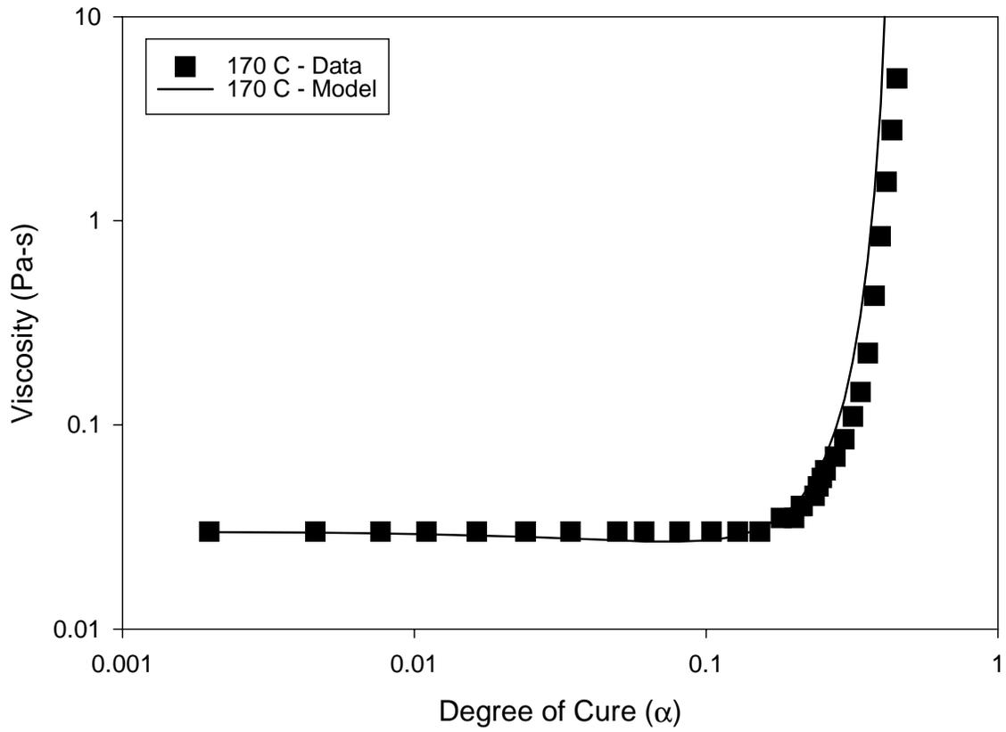
**Figure 4.8: Comparison of measured and model predicted viscosity as a function of time at 170°C for 954-3 cyanate ester resin.**
