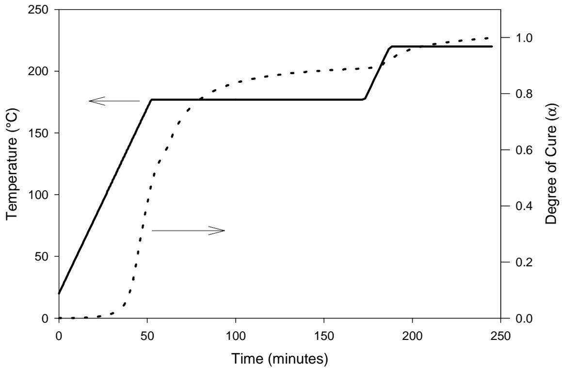
**Figure 6.4: Temperature and degree of cure as a function of time for the 954-2a cyanate ester resin flowing through the EWC-600X 8HS graphite fabric.**
