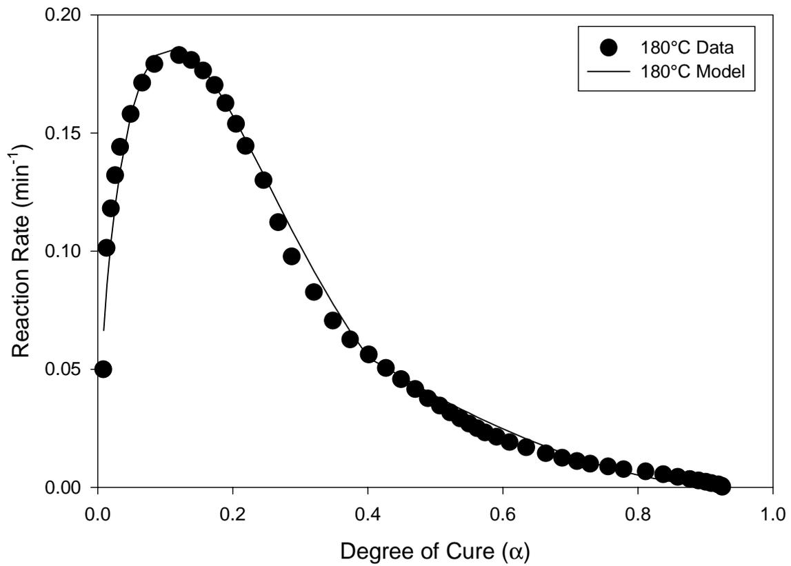
**Figure 3.33: Comparison between experimental and model values for reaction rate as a function of degree of cure for 180°C.**
