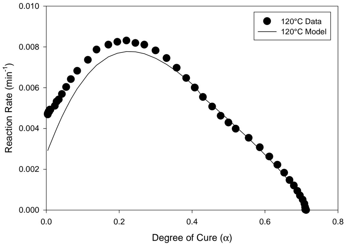
**Figure 3.39: Comparison between experimental and model values for reaction rate as a function of degree of cure for 120°C.**
