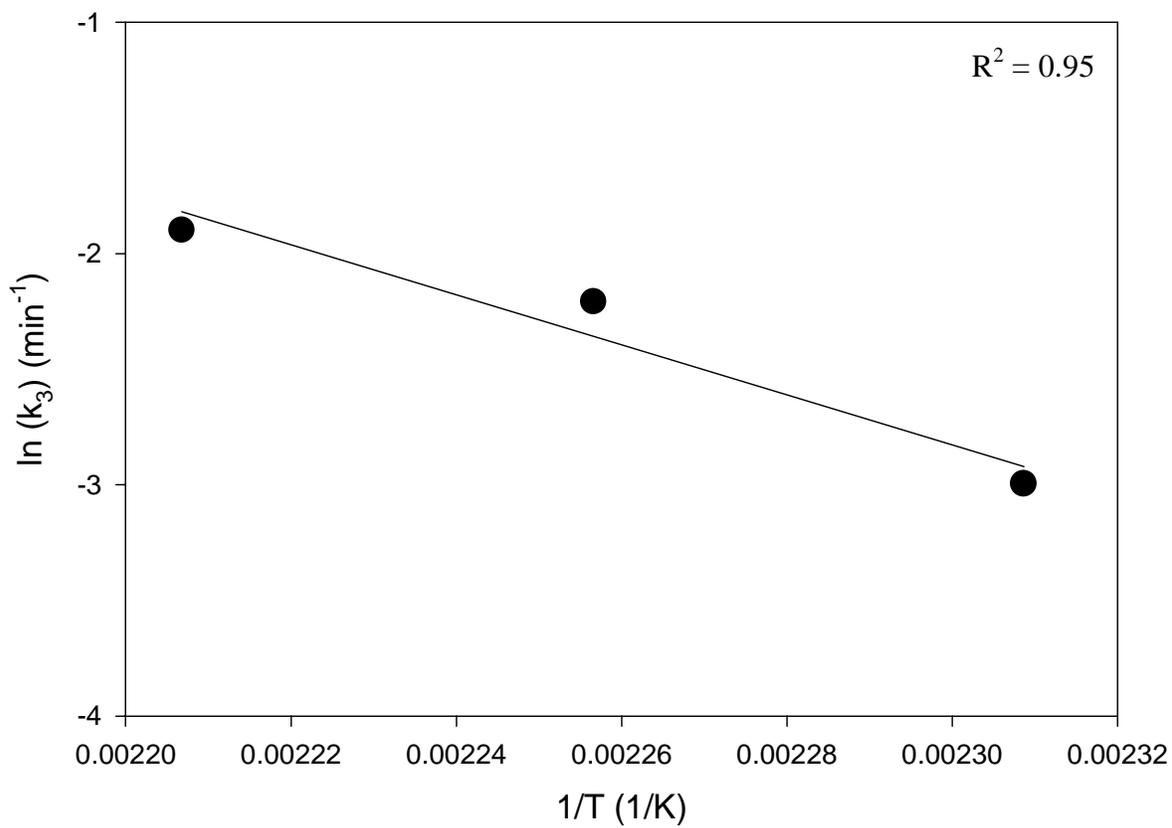
**Figure 3.22:** Plot of  $\ln(k_3)$  vs.  $1/T$  for temperatures between 160 and 180°C for Fiberite 954-2a resin.
