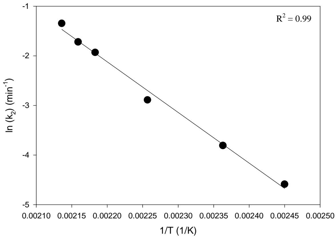
**Figure 3.8: Plot of  $\ln(k_2)$  vs.  $1/T$  for Fiberite 954-3 resin.**
