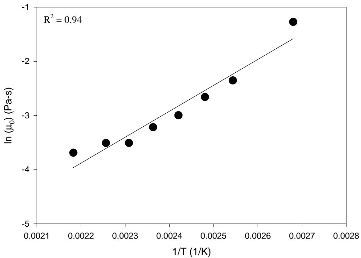
**Figure 4.2: Arrhenius plot showing the temperature dependence of initial viscosity for 954-3.**
