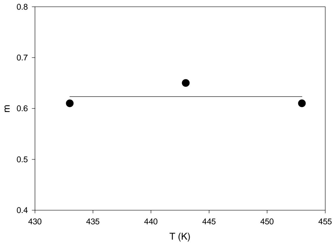
**Figure 3.23: Kinetic exponent,  $m$ , as a function of temperature between 160 and 180°C for Fiberite 954-2a resin.**
