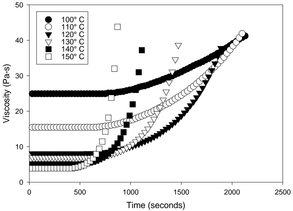
**Figure 4.10: Measured viscosity as a function of time at different isothermal temperatures for the toughened cyanate ester resin system.**
