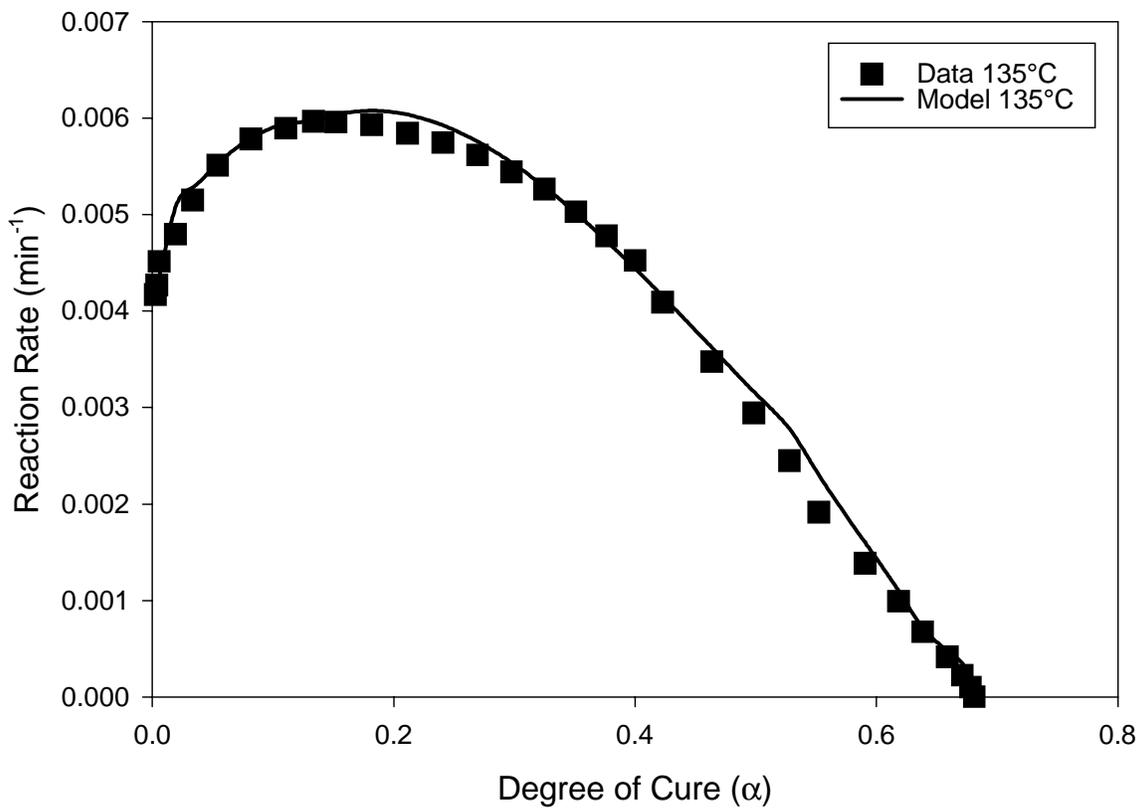
**Figure 3.19: Comparison between experimental and model values for reaction rate as a function of degree of cure for 135°C.**
