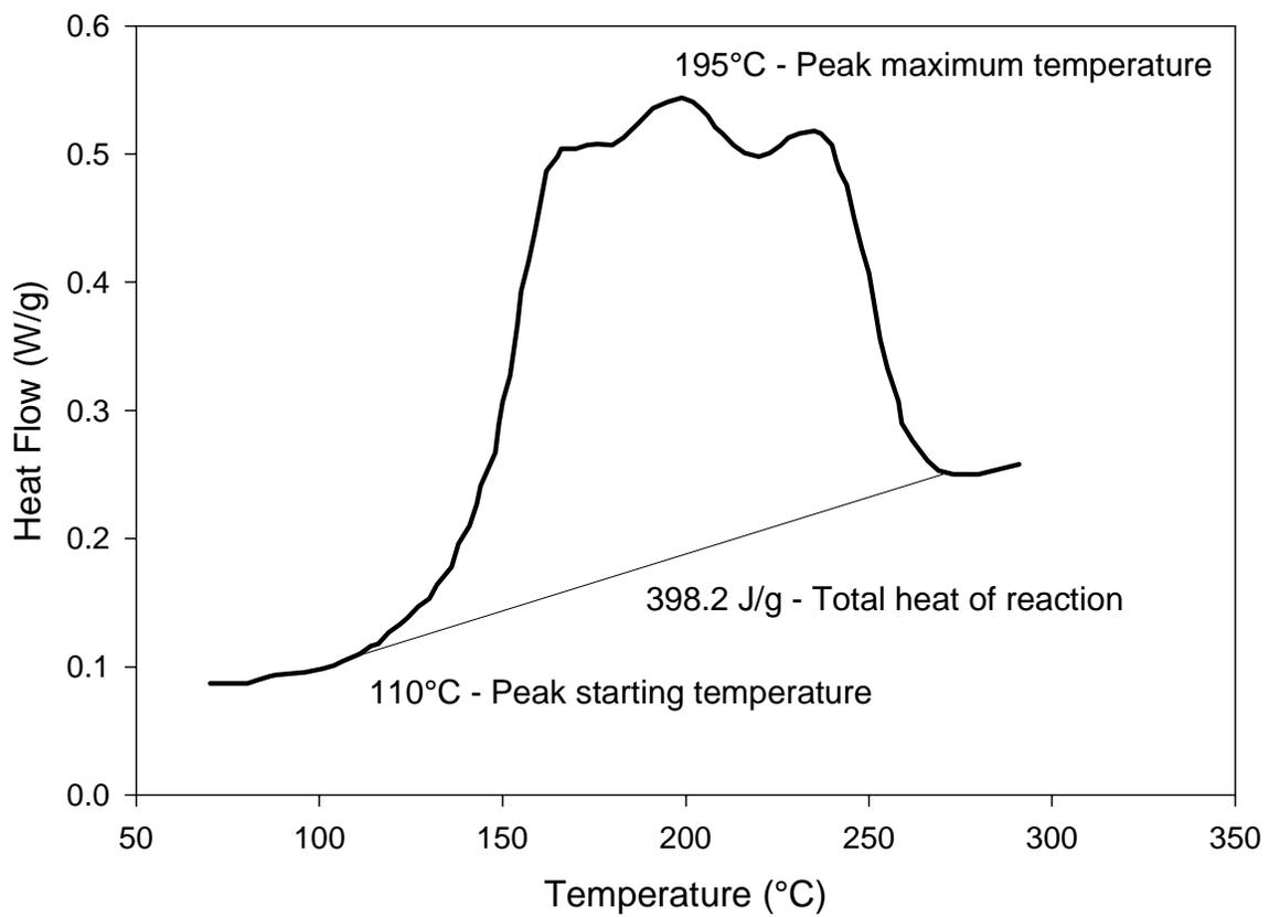
**Figure 3.1: Example dynamic scan of 954-2a run at 5°C / minute up to 300°C showing the peak starting temperature, peak maximum, and total heat of reaction.**
