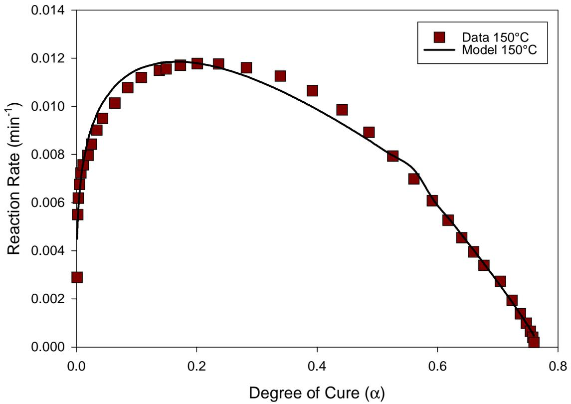
**Figure 3.18: Comparison between experimental and model values for reaction rate as a function of degree of cure for 150°C.**
