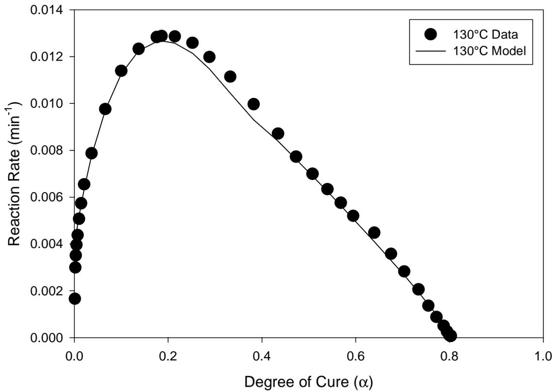
**Figure 3.38: Comparison between experimental and model values for reaction rate as a function of degree of cure for 130°C.**
