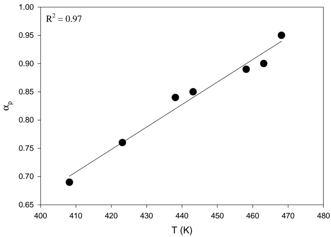
**Figure 3.13: Plot of peak degree of cure vs. temperature for Fiberite 954-3 resin.**
