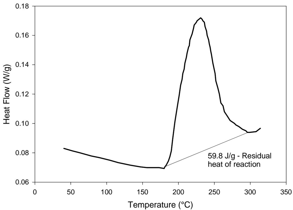
**Figure 3.3: Residual dynamic scan run at 5°C / minute immediately after the 180°C isothermal scan, showing the residual heat of reaction ( $H_{res}$ ).**
