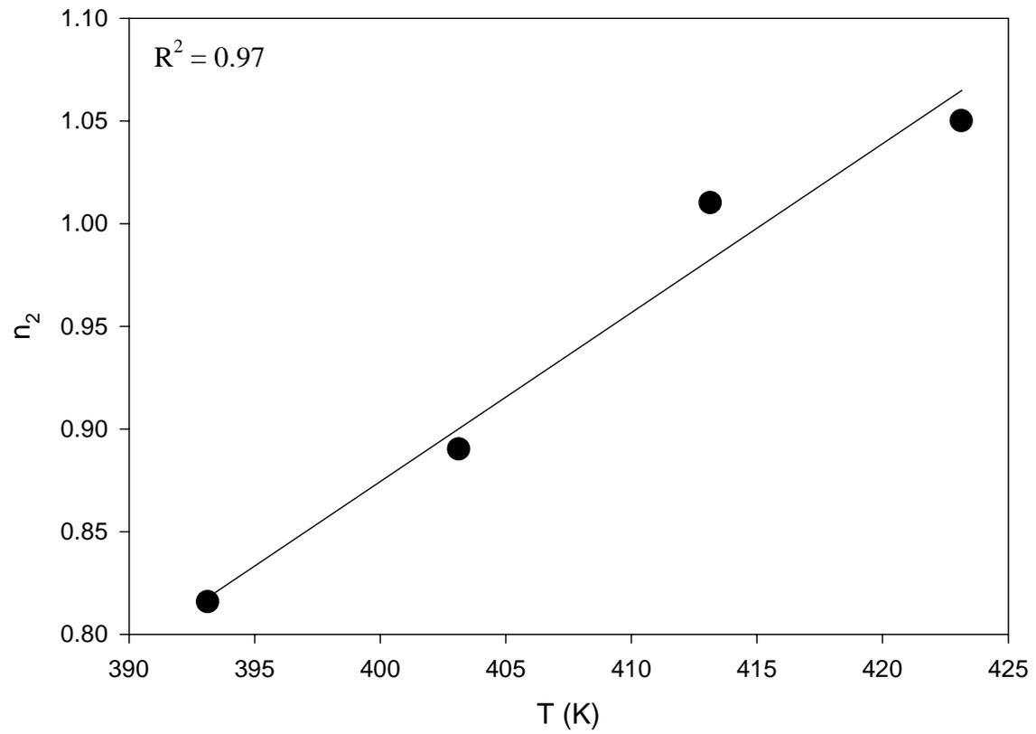
**Figure 3.31: Kinetic exponent,  $n_2$ , as a function of temperature between 120 and 160°C for Fiberite 954-2a resin.**
