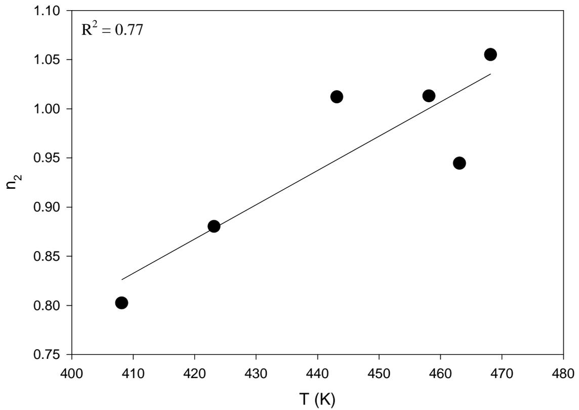
**Figure 3.12: Kinetic exponent,  $n_2$ , as a function of temperature for Fiberite 954-3 resin.**
