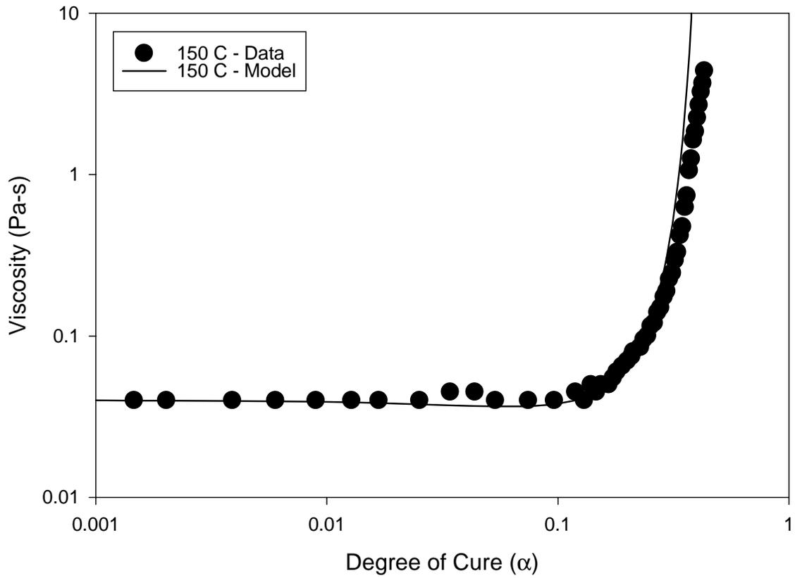
**Figure 4.7: Comparison of measured and model predicted viscosity as a function of time at 150°C for 954-3 cyanate ester resin.**
