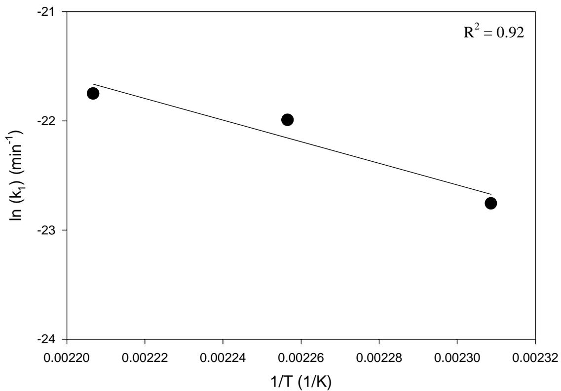
**Figure 3.20: Plot of  $\ln(k_1)$  vs.  $1/T$  for temperatures between 160 and 180°C for Fiberite 954-2a resin.**
