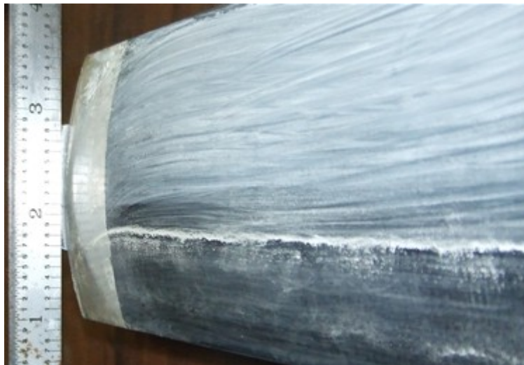
Figure 5.2B Two dimensionality from oil flow visualization
