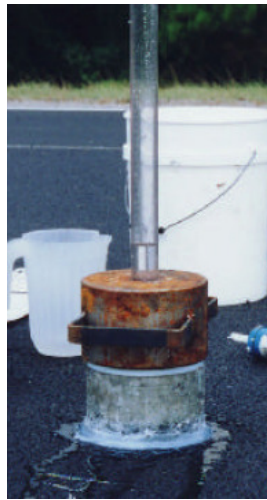
Figure 2.7 – Marshall Mold Permeameter Silicon Seal (Cooley, et al. 1999) used with permission
