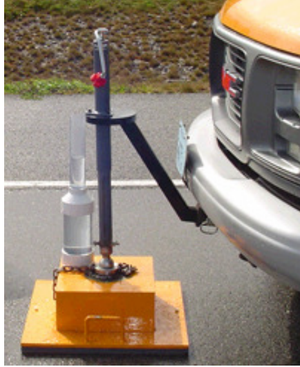
Figure 3.8 – Final Field Permeameter photographed by author
