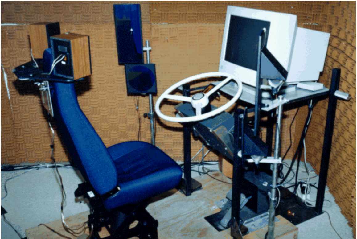
Figure 13. Side View of the commercial vehicle driving simulator facility -- participant's station.
