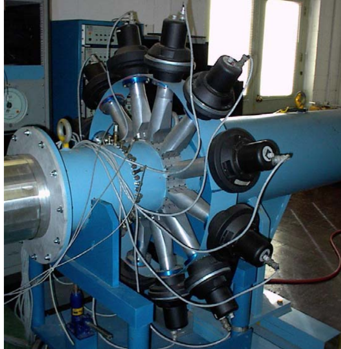
Figure 3-2: Array of 12 equally spaced acoustic drivers.
