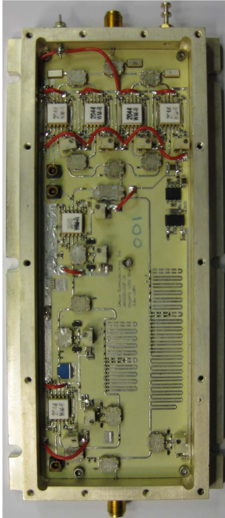
Figure 34: The built Module for the Mirror PD Linearized PA. Photo by author, 2009.
