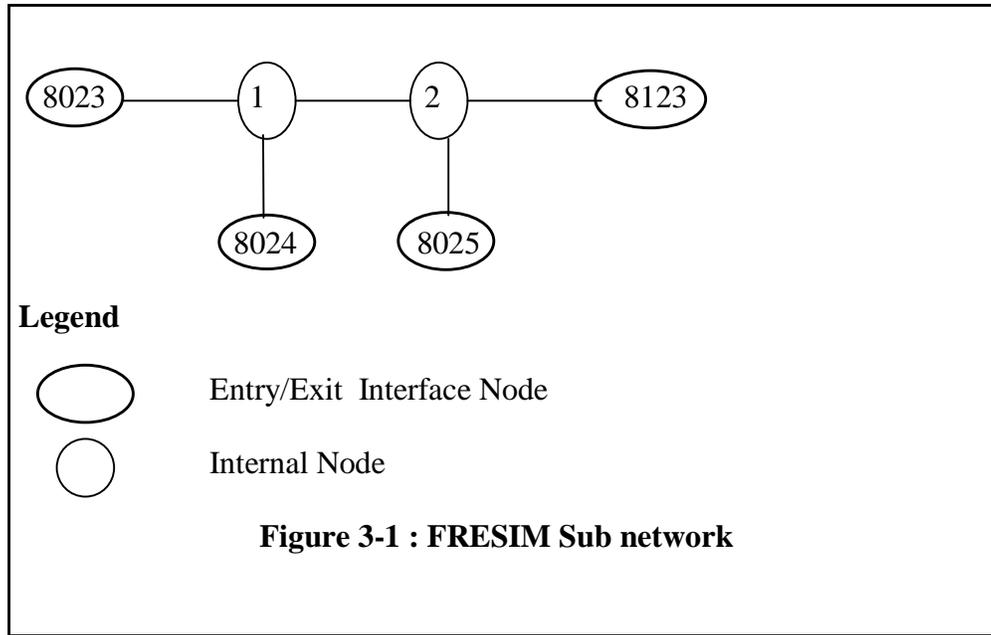
AS the name suggests CORSIM is an integration of two models i.e. NETwork SIMulation (NETSIM) and FREeway SIMulation (FRESIM). NETSIM is used to simulate local surface streets while freeway and ramp merging scenarios can be simulated using FRESIM. Since our scope of study lies within freeway simulation the description of the FRESIM model is outlined below.
