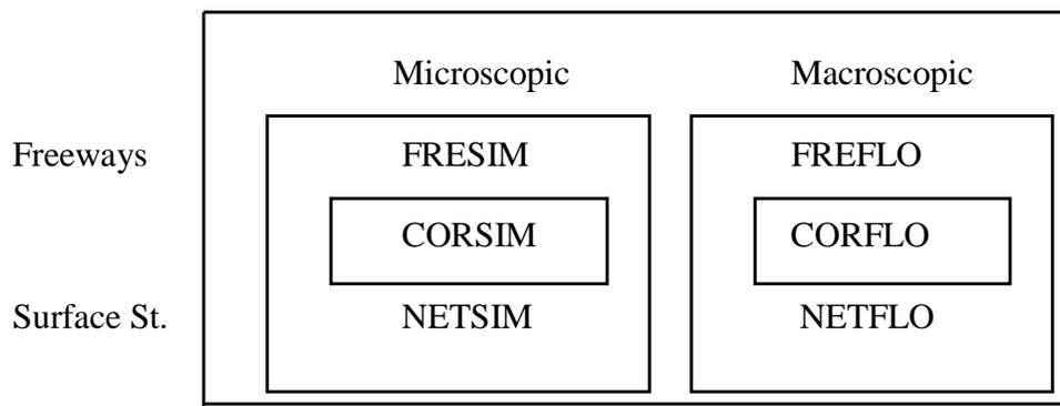
Another consideration in model selection is the intent of study. If the user is exploring traffic management concept and wishes to identify those variables that are viable candidates for more detailed analysis, CORSIM (CORridor SIMulator) would be used. In essence CORSIM and CORFLO are integrated simulation models at micro and macro simulation levels.
