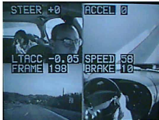
Figure 4.5. Typical quad-split image from the in-vehicle camera.
