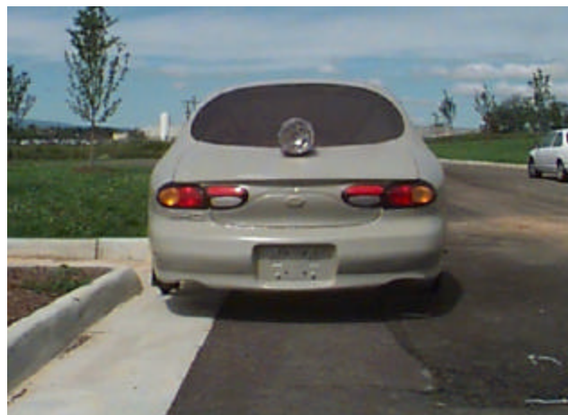
Figure 4.4. Positioning of strobe light on surrogate vehicle: rear view
