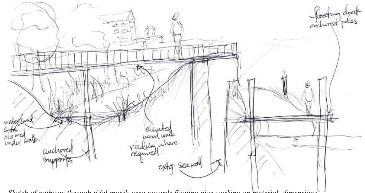
Sketch of pathway through tidal marsh area towards floating pier working on material, dimensions, and physical relationships of elements
