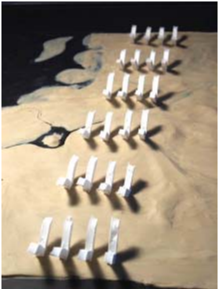
Bridge footings bisecting Jones Point and to serve as downspouts for bridge stormwater runoff
