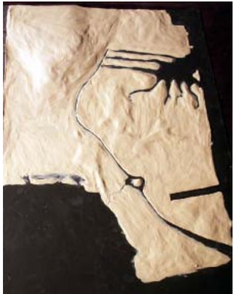
Model of Jones Point area topography with highest point northwest of site. Most of site below 8' contour and <4% slope
