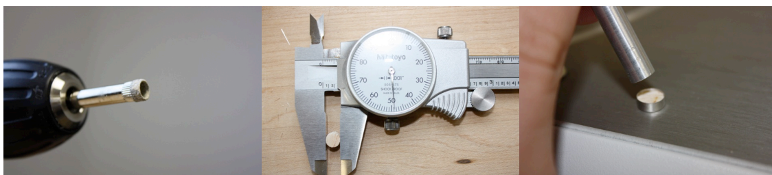
Figure 18. Core drill, STA sample, sample pushed into platinum cup
