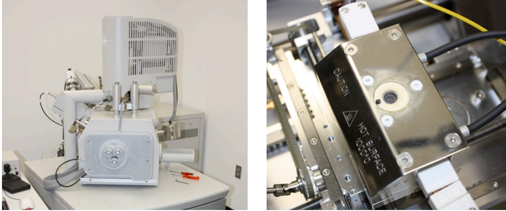
Figure 4. ESEM and internal heating platform
