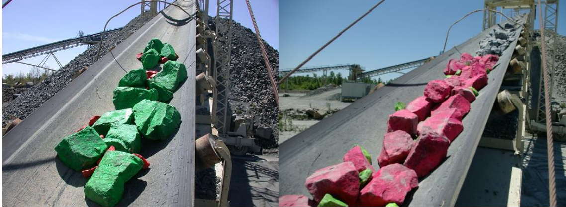
Figure 3.4 - Tracer rocks on conveyor for analysis 2 and 3, respectively
