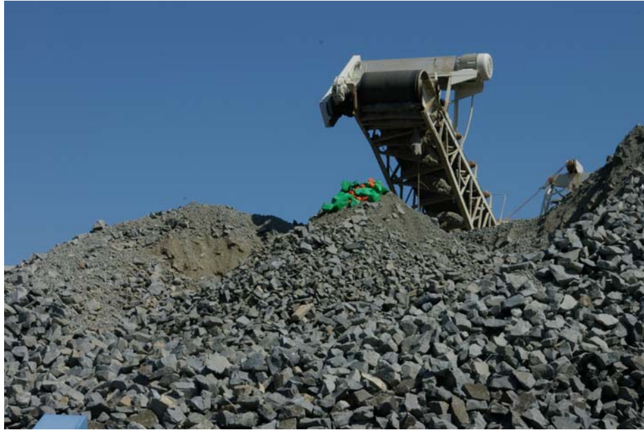
Figure 3.3 - Side view of pile (tracer rocks located at peak)
