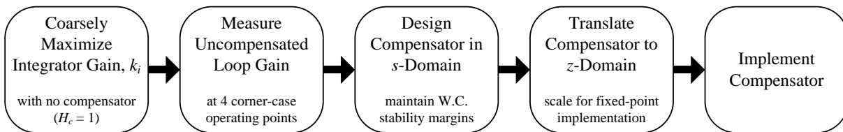
Figure 4.2 – Digital controller design process.
